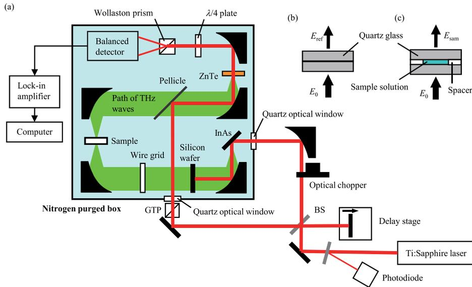
FIG. 1. Experimental setup. (a) THz-TDS system, (b) glass plates for reference, (c) structure of the sample cell. BS: Beam splitter, GTP: Glan-Taylor prism.
