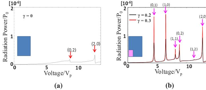
Figure 3: (color online) (a) The radiation power versus voltage ( $P$ - $V$ ) curves of the homogeneous mesa. (b) The  $P$ - $V$  curves of the inhomogeneous mesa having hot spots. The black and red lines indicate the curves for  $\gamma = 0.2$  and  $\gamma = 0.3$  respectively.
