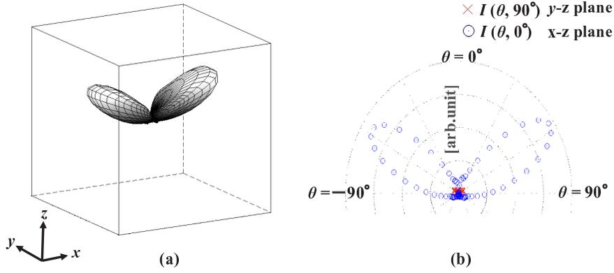
Figure 7: (color online) The radiation pattern at  $V = 12.7V_p$  in the presence of finite size substrate. (a) The three-dimensional plots of  $I(\theta, \phi)$ , and (b) The polar plots of  $I(\theta, 0^\circ)$  in the  $x$ - $z$  plane and  $I(\theta, 90^\circ)$  in the  $y$ - $z$  plane.
