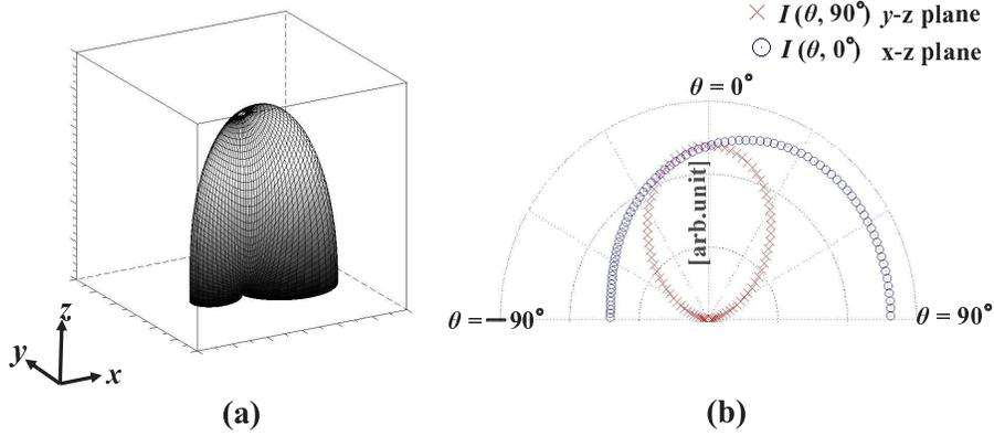
Figure 5: (color online) (a) The three-dimensional plots of the radiation intensity  $I(\theta, \phi)$  at  $V = 6.44V_p$ . (b) The polar plots of  $I(\theta, 0^\circ)$  in the  $x$ - $z$  plane and  $I(\theta, 90^\circ)$  in the  $y$ - $z$  plane at  $V = 6.44V_p$ .
