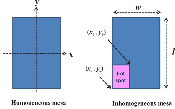
Figure 2: (color online) Schematic figures of the homogeneous mesa (left) and the inhomogeneous mesa (right).  $(x_s, y_s)$  and  $(x_e, y_e)$  are the coordinates of the two opposite corners of the hotspot.
