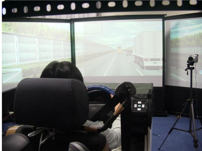
Fig. 1 The driving simulator used in the experiment
