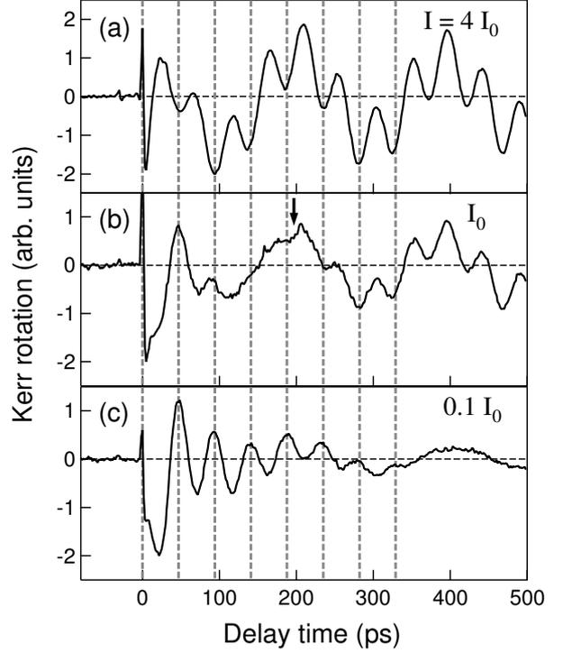
Figure 2: Experimental data of TRKR in the InP QDs, and its dependence on the pump intensity  $I$  ( $I_0 = 250$  nJ/cm<sup>2</sup>) at  $B = 1$  T and  $T = 5$  K. The vertical broken lines show the temporal points of the oscillation peaks in (c).
