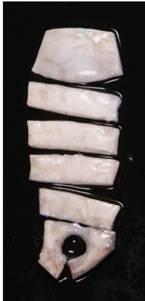
**Figure 1. Porcine sclera dissected by scalpel blades.** Strips in the lower and upper sides of the figure are peripapillary sclera and sclera near the limbus, respectively. The four strips of sclera between them were used for the measurement.
