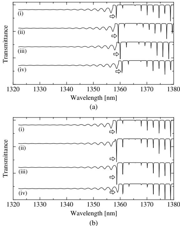
Fig. 4. Numerically simulated spectra of ring cavities modulated the refractive index of (a) the entire device and (b) only the directional coupler. The spectra are varied from (i) to (iv) by the modulation. The resonance peak of the identical ring resonance mode is indicated by arrows. The widths of the resonance peaks for (a) are hardly varied, while those for (b) are varied, with their peak position fixed.
