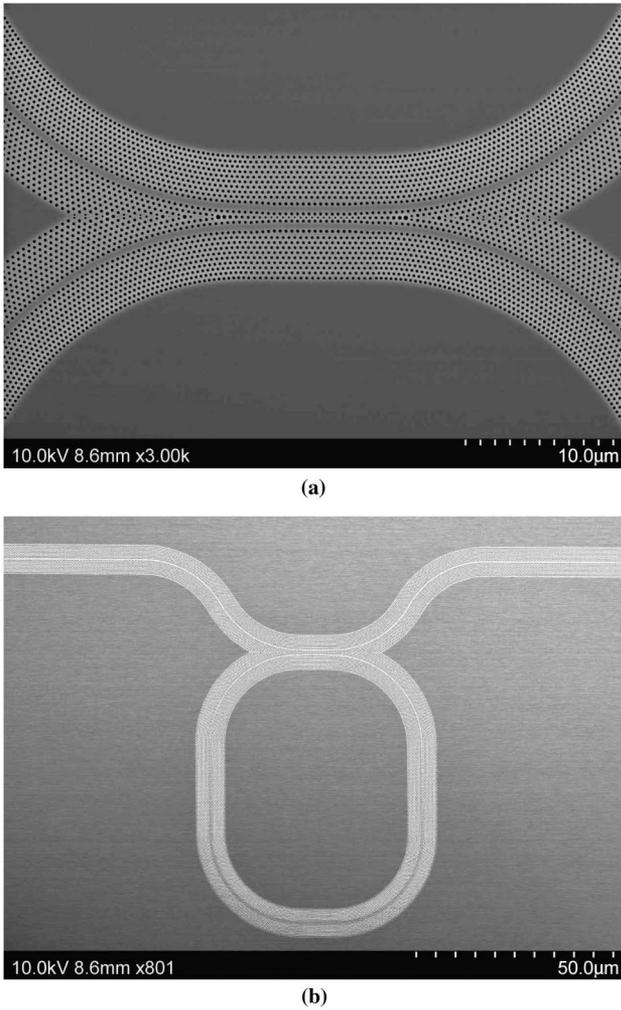
Fig. 2. Surface SEM images of the (a) entire microring cavity and (b) flat-band directional coupler. The length of the ring waveguide is  $520a$  with a curvature of  $1.0^\circ/a$ . The length of the flat-band directional coupler is  $12a$ . Both ends are connected to a  $5a$  long adiabatic connector.
