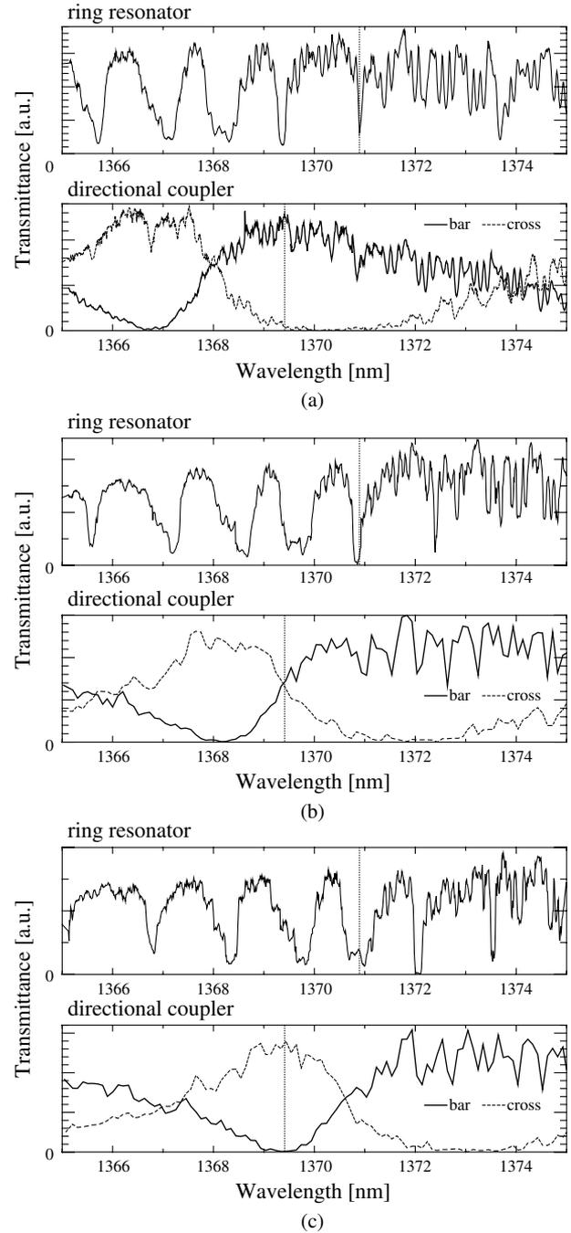
Fig. 3. Transmission spectra of the ring cavity (left side) and directional coupler (right side) at (a) 25.2°C, (b) 50.0°C, and (c) 68.8°C. The width of the resonance peak depends on the state of the directional coupler; broad peaks corresponds to the cross state, and sharp peaks correspond to the bar state. As the temperature is increased, the spectra are redshifted and the peak at 1370.9 nm (indicated by vertical dashed lines) becomes sharp.
