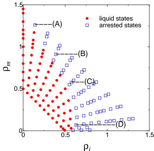
**Figure 2.** Dynamic phase diagram of the binary soft-core mixture generated by the EM protocol.  $\rho_i$  is the immobile (obstacle) particle density, and  $\rho_m$  is the mobile (fluid) particle density. The arrested states are defined as the points beyond which the  $\alpha$ -relaxation time  $\tau_\alpha$  exceeds  $10^3$ .
