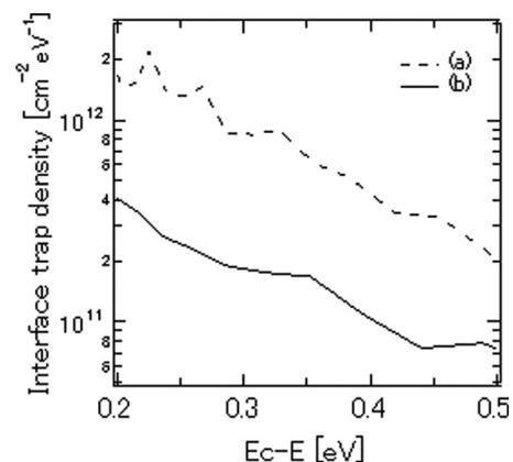
FIG. 2. Comparison of  $D_{it}$  for n-type MOS capacitors formed (a) without and (b) with nitridation at 1467 °C for 5 min. A gate oxide layer was formed by PECVD. Both MOS capacitors were etched in HF just before oxide deposition.
