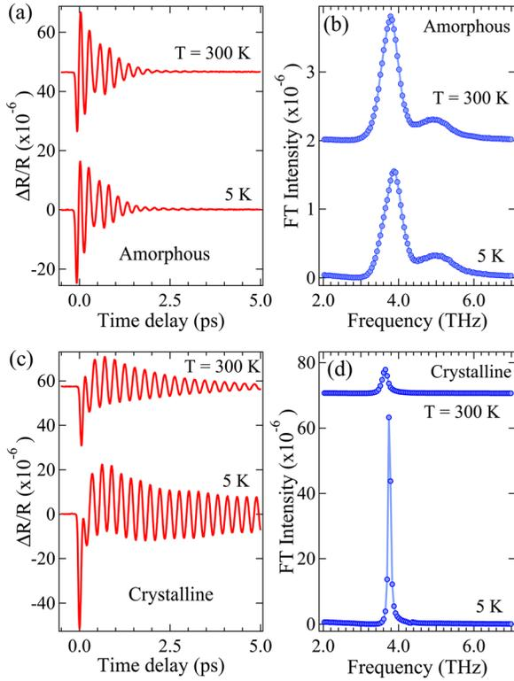
FIG. 1. (Color online). (a) and (c) The time-resolved TR signal observed at 5 and 300 K in the *a*- and *c*-GeTe/Sb<sub>2</sub>Te<sub>3</sub> SL films, respectively. (b) and (d) The FT spectra obtained from the time-domain data in (a) and (c).
