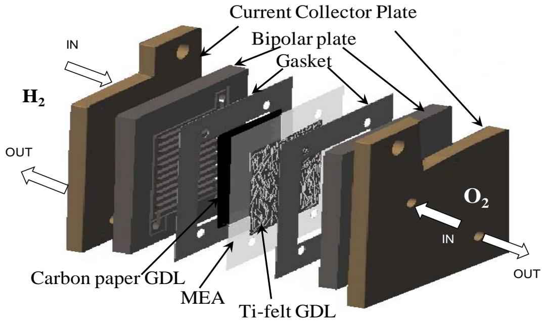
Figure 1. Schematic of a URFC with single-cell structure.
