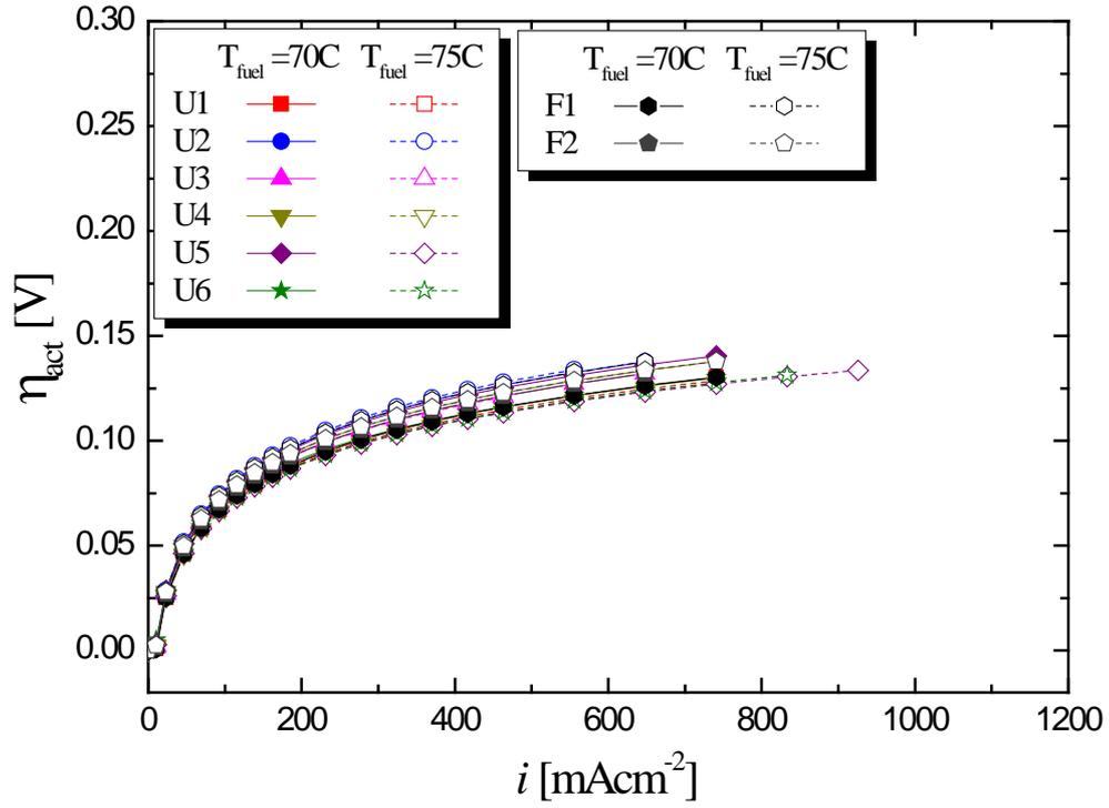
**Figure 9.** Current density ( $i$ ) - activation overpotential ( $\eta_{act}$ ) characteristics during fuel cell mode for U1~U6 and F1 and F2 cells at humidification temperature ( $T_{fuel}$ ) of 70 and 75°C. Cell temperature ( $T_{cell}$ ) was 80°C.
