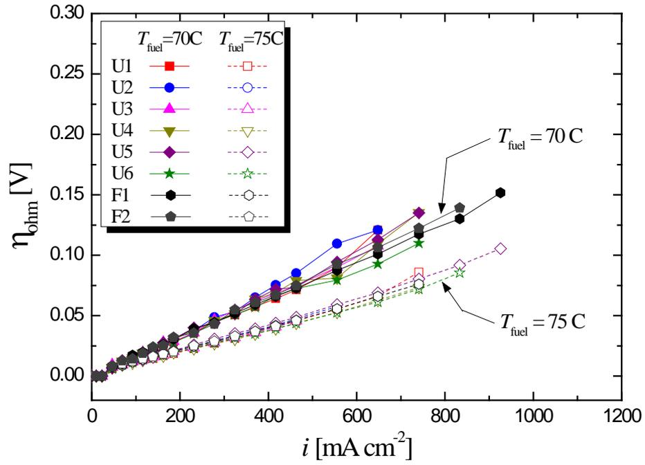
**Figure 10.** Current density ( $i$ ) - ohmic overpotential ( $\eta_{ohm}$ ) characteristics during fuel cell mode for U1~U6 and F1 and F2 cells at humidification temperature ( $T_{fuel}$ ) of 70 and 75°C. Cell temperature ( $T_{cell}$ ) was 80°C.
