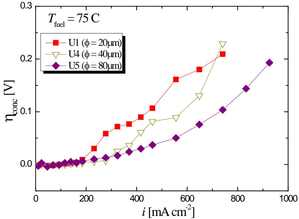
**Figure 16.** Effect of fiber diameter ( $\phi$ ) of the Ti-felt GDL of the oxygen electrode on the current density ( $i$ ) - concentration overpotential ( $\eta_{\text{conc}}$ ) characteristics during fuel cell mode for U1, U4, and U5 cells (with no PTFE treatment) at humidification temperature ( $T_{\text{fuel}}$ ) of 75°C. Cell temperature ( $T_{\text{cell}}$ ) was 80°C.  $\eta_{\text{conc}}$  was calculated from the  $i$ - $V$  data shown in Fig. 15(B).
