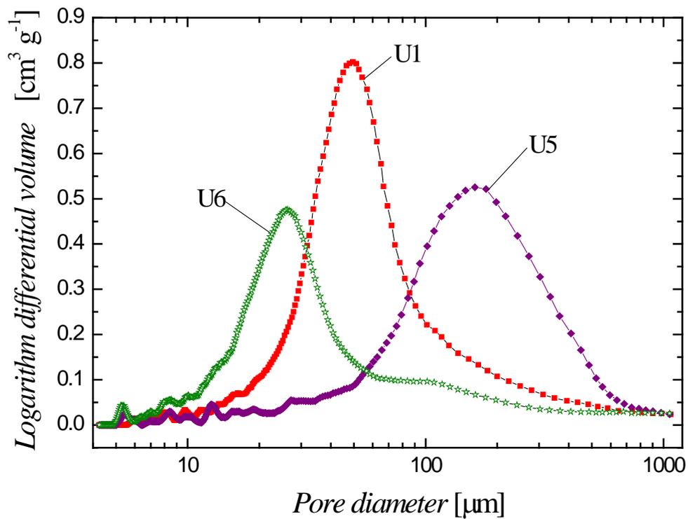
**Figure 6.** Pore volume distribution in Ti-felt GDL substrates used in U1, U5, and U6 represented by pore diameter and logarithm of the differential volume ( $= dV / d \log(d)$ ) measured using a mercury intrusion porosimeter (MIP).
