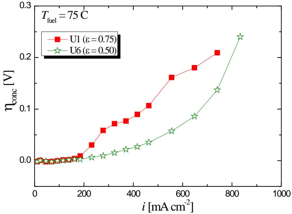
**Figure 18.** Effect of porosity ( $\epsilon$ ) of the Ti-felt GDL of the oxygen electrode on the current density ( $i$ ) - concentration overpotential ( $\eta_{\text{conc}}$ ) characteristics during fuel cell mode for U1 and U6 cells at humidification temperature ( $T_{\text{fuel}}$ ) of 75°C. Cell temperature ( $T_{\text{cell}}$ ) was 80°C.  $\eta_{\text{conc}}$  was calculated from the  $i$ - $V$  data shown in Fig. 17(B).
