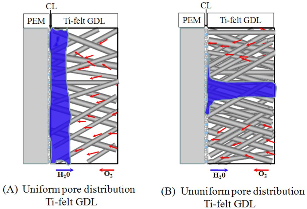
**Figure 19.** Schematic of liquid water and air transport for different Ti-felt GDL substrates (A) with uniform pore distribution structure as in U1 (B) with ununiform pore distribution pore distribution as in U4, U5, and U6.
