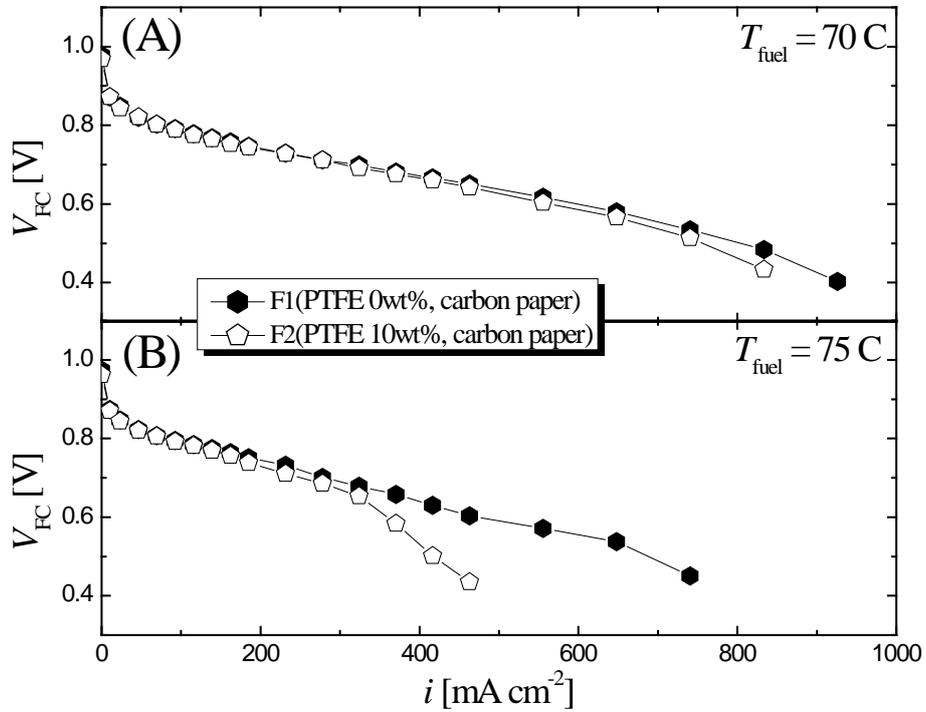
**Figure 13.** Effect of PTFE content in carbon-paper GDL substrates of the oxygen electrode on current density ( $i$ ) - voltage ( $V$ ) characteristics during fuel cell mode for F1 and F2 cells at humidification temperature ( $T_{\text{fuel}}$ ) of (A) 70°C and (B) 75°C, The carbon paper GDL of the oxygen electrode is not treated with PTFE in F1, and the one is treated with 10wt.% PTFE emulsion in F2. when the cell temperature is 80°C.
