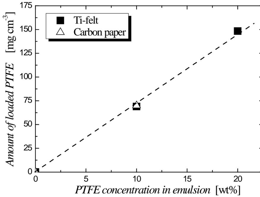
**Figure 3.** Relation between PTFE concentration in emulsion and amount of PTFE loaded on GDL substrates of Ti-felt and carbon paper.
