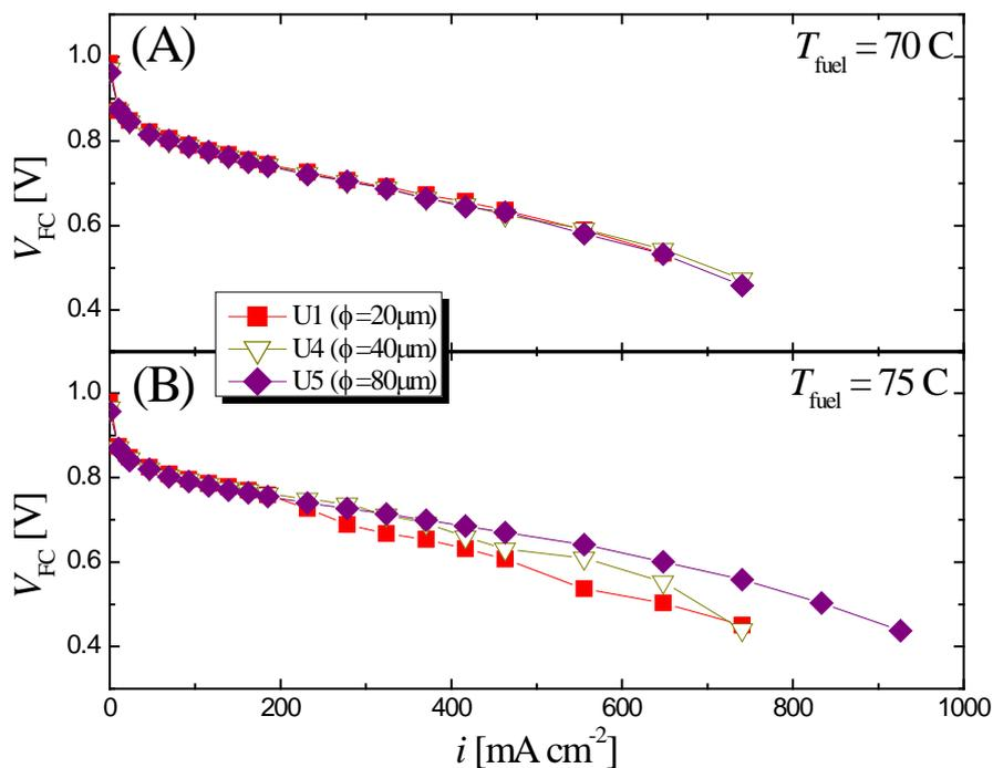
**Figure 15.** Effect of fiber diameter ( $\phi$ ) of the Ti-felt GDL of the oxygen electrode on the current density ( $i$ ) - voltage ( $V$ ) characteristics during fuel cell mode for U1, U4, and U5 cells (with no PTFE treatment) at humidification temperature ( $T_{fuel}$ ) of (A)  $70\text{ C}$  and (B)  $75\text{ C}$ . Cell temperature ( $T_{cell}$ ) was  $80\text{ C}$ .
