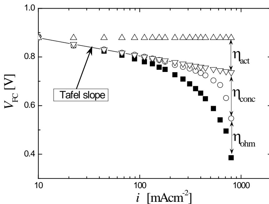
**Figure 4.** Polarization curves and overpotential separation into activation overpotential ( $\eta_{act}$ ), ohmic overpotential ( $\eta_{ohm}$ ), and concentration overpotential ( $\eta_{conc}$ ), during fuel cell mode for a Ti-felt GDL of the oxygen electrode without PTFE treatment.
