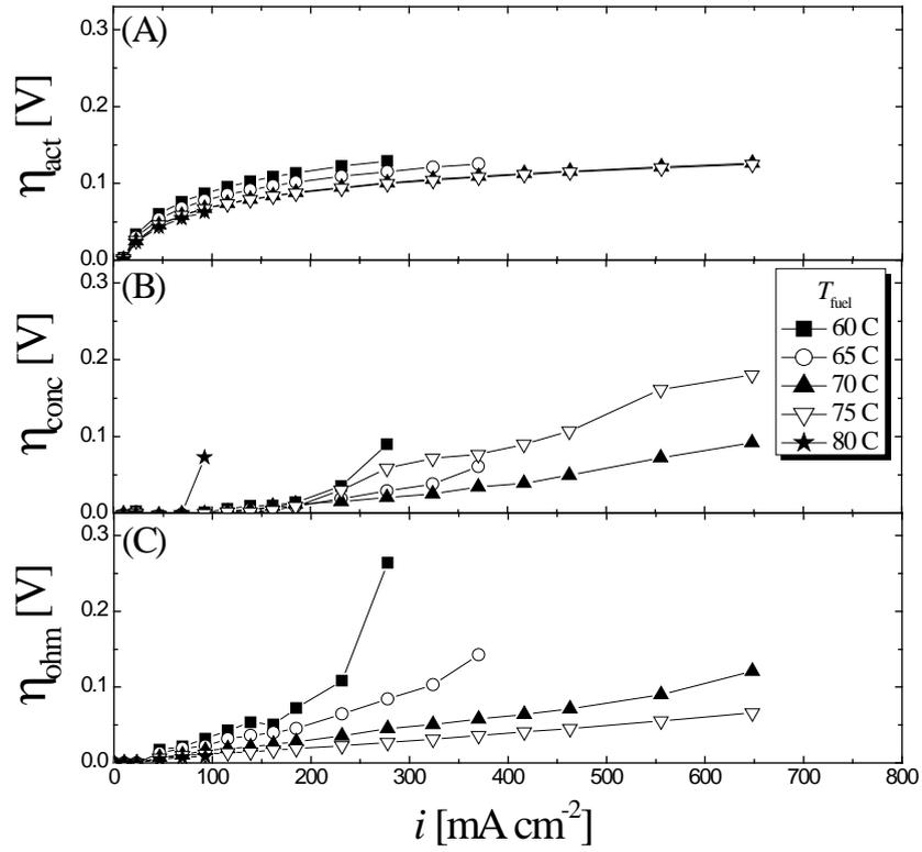
**Figure 8.** Effect of humidification temperature ( $T_{\text{fuel}}$ ) on current density ( $i$ ) and overpotential characteristics for (A) activation overpotential ( $\eta_{\text{act}}$ ), (B) concentration overpotential ( $\eta_{\text{conc}}$ ), and (C) ohmic overpotential ( $\eta_{\text{ohm}}$ ) during fuel cell mode with U1 cell. Cell temperature ( $T_{\text{fuel}}$ ) was 80°C.
