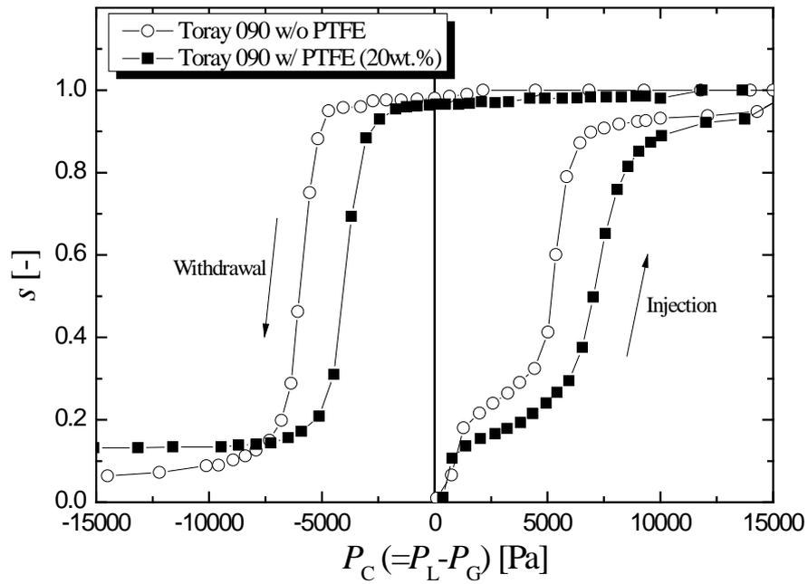
**Figure 14.** Liquid water saturation ( $s$ ) versus capillary pressure ( $P_c$ ) characteristics with the Toray 090 substrate presented by Gostick et al. [34], ( $-\circ-$ ): Toray 090 without PTFE treatment. ( $-\blacksquare-$ ): Toray 090 with PTFE 20wt.%.
