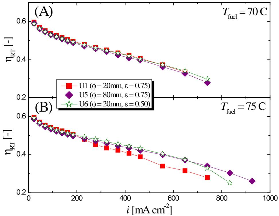
**Figure 20.** Effect of fiber diameter ( $\phi$ ) and porosity ( $\epsilon$ ) of Ti-felt GDLs on the current density ( $i$ ) and round-trip efficiency ( $\eta_{RT}$ ) during electrolysis and fuel cell modes for U1, U5, and U6 cells at humidification temperature ( $T_{\text{fuel}}$ ) of (A) 70 and (B) 75°C. Cell temperature ( $T_{\text{cell}}$ ) was 80°C.
