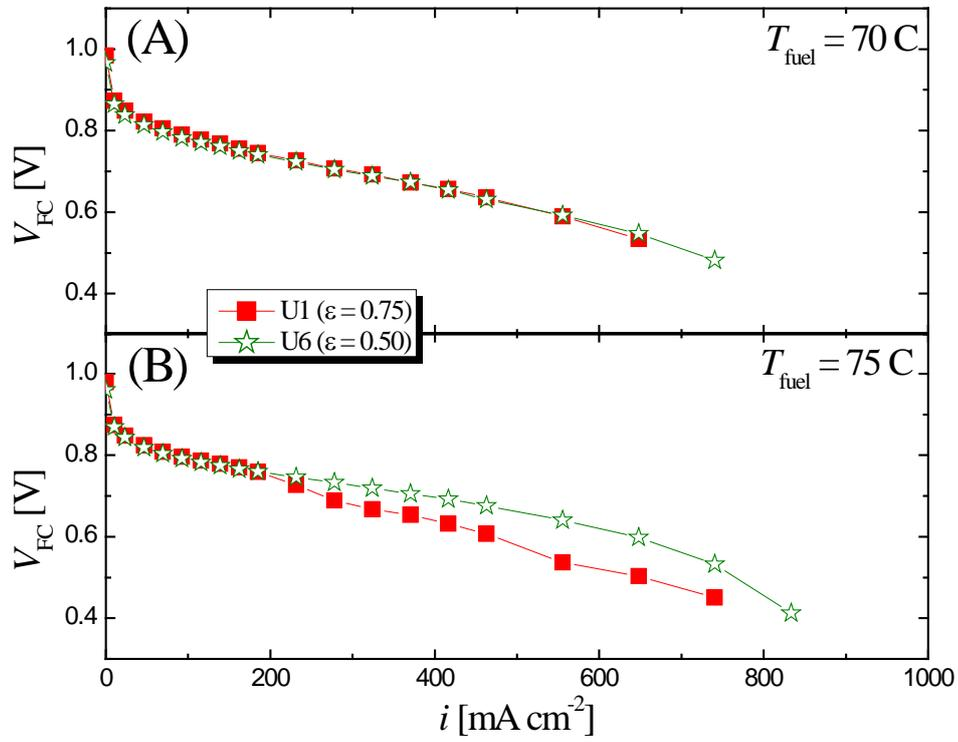
**Figure 17.** Effect of porosity ( $\epsilon$ ) of the Ti-felt GDL of the oxygen electrode on the current density ( $i$ ) - voltage ( $V$ ) characteristics during fuel cell mode for U1 and U6 cells at humidification temperature ( $T_{\text{fuel}}$ ) of (A)  $70^{\circ}\text{C}$  and (B)  $75^{\circ}\text{C}$ . Cell temperature ( $T_{\text{cell}}$ ) was  $80^{\circ}\text{C}$ . The Ti-felt GDLs were not treated with PTFE, and had fiber diameter ( $\phi$ ) of  $20\mu\text{m}$ .
