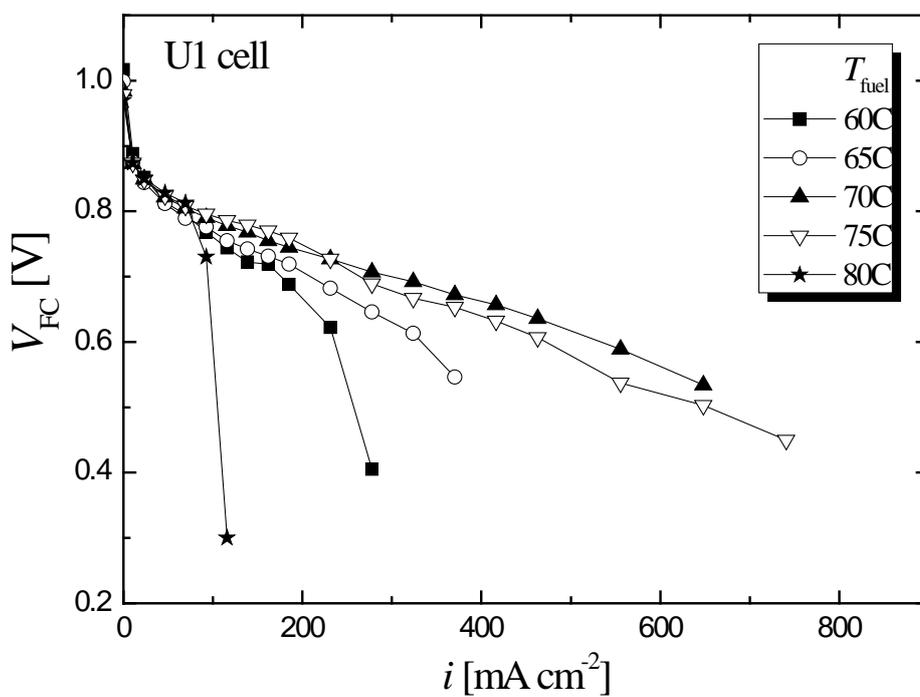
**Figure 7.** Effect of humidification temperature ( $T_{\text{fuel}}$ ) of gases ( $\text{H}_2$  and air) on current density ( $i$ ) and voltage ( $V$ ) characteristics during fuel cell mode of the U1 cell. In the U1 cell, the hydrogen-side GDL was carbon paper treated with 10 wt% PTFE, and the oxygen-side GDL was Ti-felt without PTFE treatment. Cell temperature ( $T_{\text{cell}}$ ) was 80°C.
