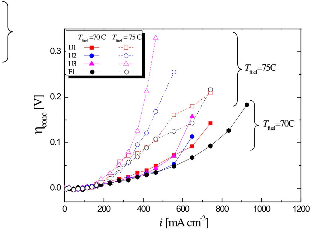
**Figure 12.** Effect of PTFE content in Ti-felt GDL substrates of the oxygen electrode on current density ( $i$ ) - concentration overpotential ( $\eta_{\text{conc}}$ ) characteristics during fuel cell mode for U1, U2, U3, and F1 cells at humidification temperature ( $T_{\text{fuel}}$ ) of 70 and 75°C. Cell temperature ( $T_{\text{cell}}$ ) was 80°C.  $\eta_{\text{conc}}$  was calculated from the  $i$ - $V$  data shown in Fig. 11.
