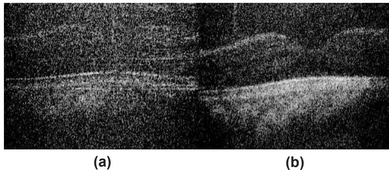
Fig. 5. Image comparison between the integration times of (a)  $1 \text{ ms}$  and (b)  $311 \mu\text{s}$ . The fringe washout affects the entire cross-sectional image. The shown representative image is 29th one in 256 successively captured cross-sectional image. A movie of the time sequence of the images are available for the comparison between with integration times of  $1 \text{ ms}$  and  $311 \mu\text{s}$  (2.1 MB movie). Also, a version of 8.0 MB is available.
