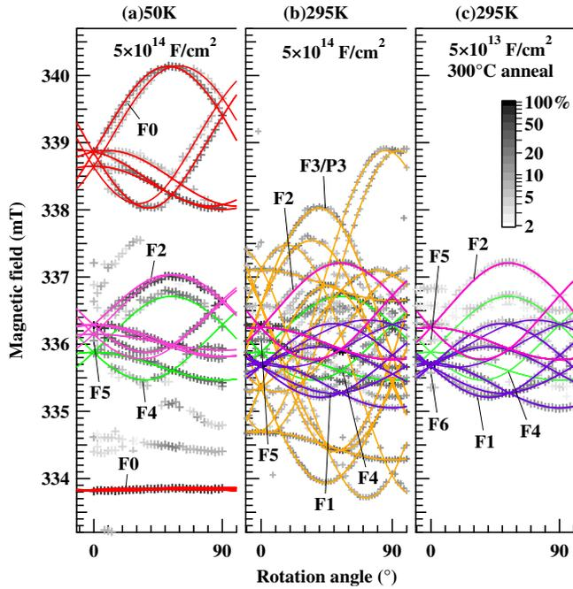
FIG. 2. (Color online) Angular maps of F0–F4 centers ( $F_nV_m$  defects) at 9.437 GHz. Magnetic field was rotated from [100] ( $0^\circ$ ) to [011] ( $90^\circ$ ). Gray symbols indicate experimental peak positions and their normalized intensities (the largest peak=100%) are expressed by a gray scale shown in inset. Solid lines are simulated by SH parameters in Table I. There are still untraced angular maps (e.g., F5 and F6), suggesting more variety of minor  $F_nV_m$  defects.
