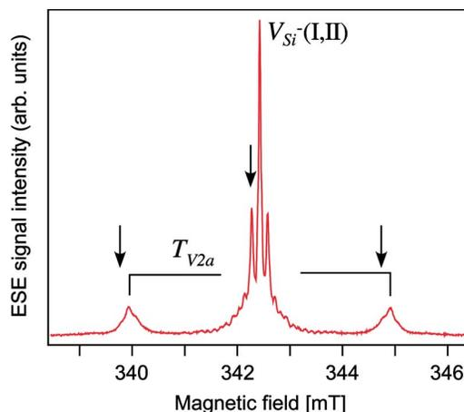
FIG. 1. (Color online) ESE spectrum of the electron-irradiated  $n$ -type  $4H$ -SiC at room temperature taken with the magnetic field along the  $c$  axis ( $[0001]$  axis). The microwave frequency was  $\nu = 9.599$  GHz. The arrows indicate the magnetic field positions where the ENDOR spectra were measured.
