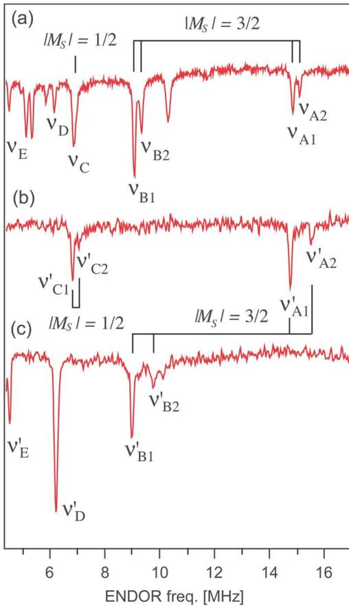
FIG. 2. (Color online) ENDOR spectrum the electron-irradiated *n*-type 4H-SiC at room temperature taken with the magnetic field along the *c* axis ([0001] axis). (a) Spectrum of  $V_{Si}^{-}(I,II)$  at 342.3 mT. (b) Spectrum of  $T_{V2a}$  at low-field side (339.8 mT). (c) The spectrum of  $T_{V2a}$  at high-field side (344.8 mT).
