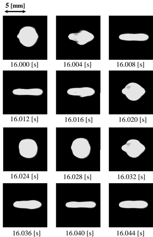
Fig. 8: Typical snapshots of oscillation of a levitated droplet (equivalent diameter: 4 mm, sound pressure: 4.0 kPa, input energy: 0.76 W)
