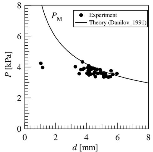
Fig. 2: Correlation between the sound pressure and the equivalent droplet diameter under the stably-levitated condition
