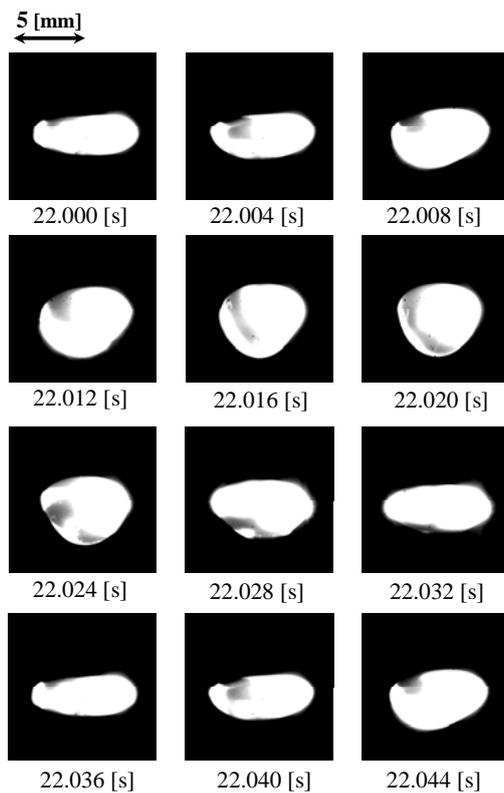
Fig. 6: Typical snapshots of oscillation of a levitated droplet (equivalent diameter: 5.5 mm, sound pressure: 3.6 kPa, input energy: 1.58 W)
