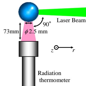
(b) Temperature measurement of a droplet surface
