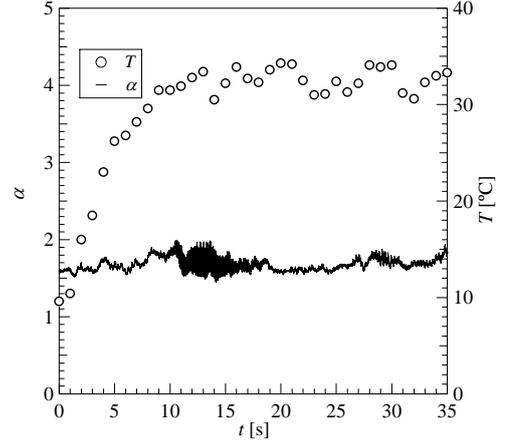
Fig. 4: Time variation of aspect ratio and temperature of levitated water droplet (equivalent diameter: 4 mm, sound pressure: 3.6 kPa, input energy: 0.76 W)
