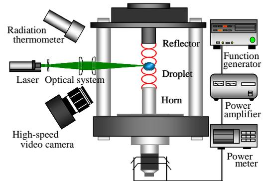
(a) Ultrasonic levitator and measurement equipment
