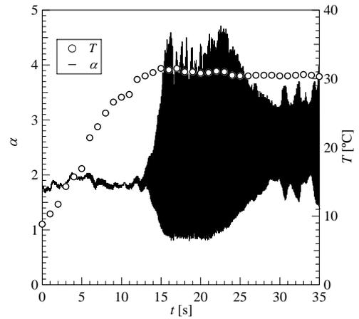
Fig. 7: Time variation of aspect ratio and temperature of levitated water droplet (equivalent diameter: 4 mm, sound pressure: 4.0 kPa, input energy: 0.76 W)
