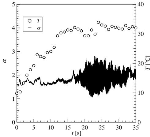
Fig. 5: Time variation of aspect ratio and temperature of levitated water droplet (equivalent diameter: 5.5 mm, sound pressure: 3.6 kPa, input energy: 1.58 W)
