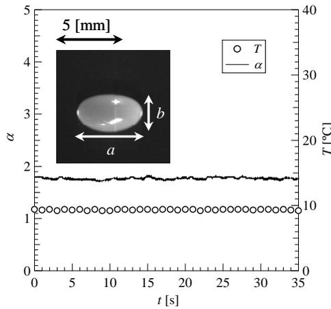
Fig. 3: Time variation of aspect ratio and temperature of non-heated levitated water droplet (equivalent diameter: 4 mm, sound pressure: 3.6 kPa, input energy: 0.0 W)
