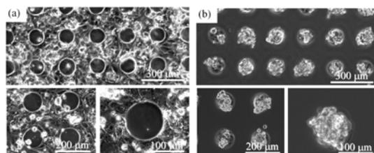
**Fig. 4** Phase-contrast micrographs of the FLC-4 sheet with 100 μm aligned cavity structure and cell spheroid array. FLC-4 cultured on a PEG gel pattern surface prepared by (a) Method A and (b) Method B. Experimental conditions are described in ESI.
