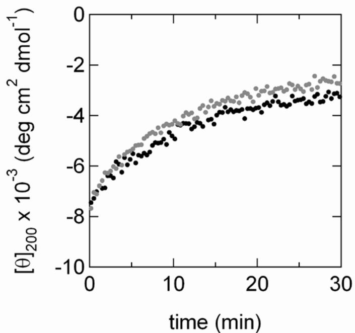
**Figure 6.** Time course of structural change of 0.1 mg/ml HN in the absence and presence of 0.17 mM DOPC in 10 mM of sodium phosphate buffer, pH7.0. Black and gray symbols were taken in the presence and absence of DOPC. CD signal at 200 nm was monitored as a function of temperature.
