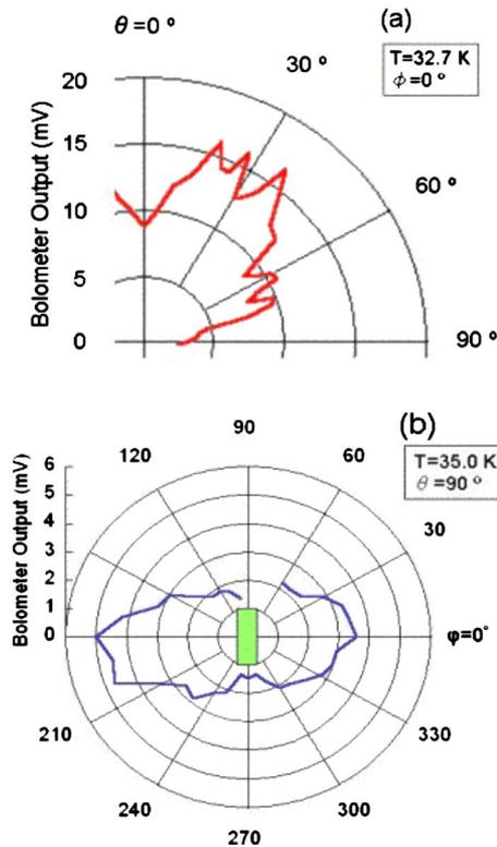
FIG. 3. (Color online) Spatial distribution of the emission from a mesa of BSCCO. The data were taken with an intensity accuracy of about 0.5 mV without a Si hemispherical lens. (a) The  $\theta$  dependence of the emission intensity at  $\varphi=0^\circ$  and (b) the  $\varphi$  dependence at  $\theta=90^\circ$ , with the angle resolution of  $4.3^\circ$ .
