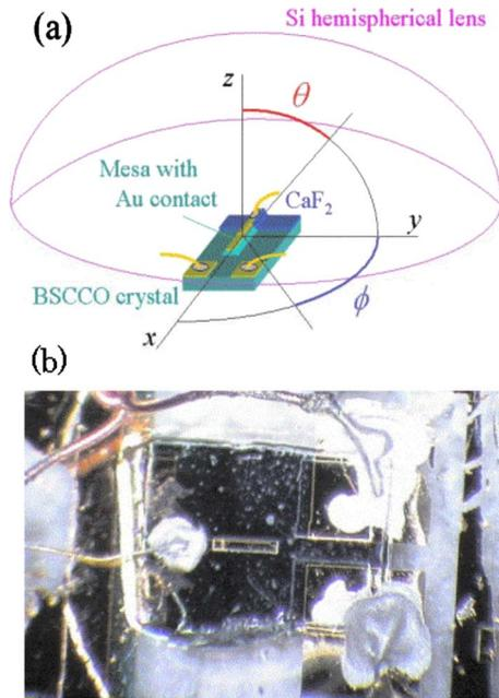
FIG. 1. (Color online) Sample arrangement. The  $(x, y, z)$  coordinates and the angles  $\theta$  and  $\phi$  are defined on the mesa as shown in (a). (b) A photograph of the BSCCO mesa used for the present experiment.
