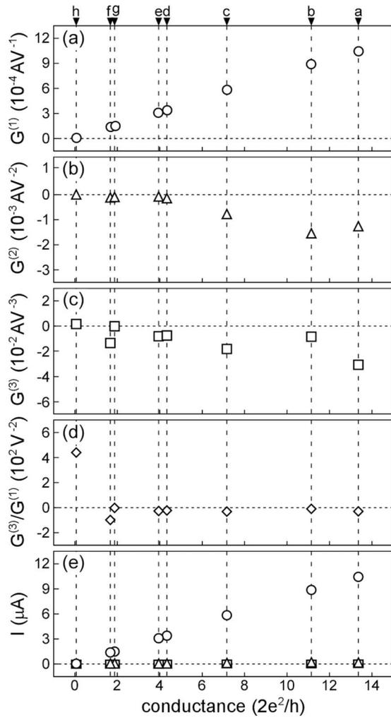
FIG. 11. Coefficients of polynomials ( $I_{\text{total}}=G^{(1)}V+G^{(2)}V^2+G^{(3)}V^3$ ;  $I_{\text{total}}$ : total current;  $V$ : bias voltage;  $G^{(1)}$ ,  $G^{(2)}$ , and  $G^{(3)}$  are coefficients of the first-, second-, and third-order terms) fitting the current-voltage curves of the contact presented in Figs. 7(a)–7(h), the ratio  $G^{(3)}/G^{(1)}$ , and  $I$  of  $G^{(1)}V$ ,  $G^{(2)}V^2$ , and  $G^{(3)}V^3$  against conductance.
