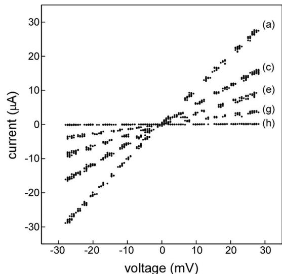
FIG. 10. Current-voltage curves of the nanocontact and single-atom-width wire presented in Figs. 7(a), 7(c), 7(e), 7(g), and 7(h). The conductance at  $0$  V is  $13$ ,  $7.5$ ,  $3.9$ ,  $2.0$ , and  $0.1G_0$  for curves (a), (c), (e), (g), and (h), respectively.
