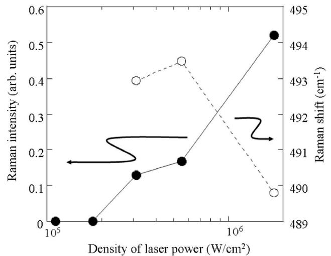
FIG. 5. Increment of Raman peak intensity (closed circles) of Si optical phonon after 532 nm cw laser irradiation, depending on power density of  $1.1 \times 10^5\text{--}1.8 \times 10^6\text{ W cm}^{-2}$  and Raman shift of Si optical phonon during cw laser irradiation (open circles).
