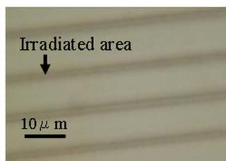
FIG. 2. (Color online) Optical image of drawn lines formed inside  $\text{SiO}_2$  substrate near Al/ $\text{SiO}_2$  interface by femtosecond-laser scanning with  $\sim 4 \times 10^3$  shots.
