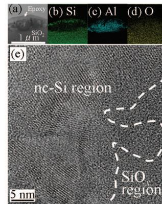
FIG. 3. (Color) Bright-field cross-section scanning TEM images (a) of Al-doped  $\text{SiO}_x$  region by femtosecond-laser irradiation and corresponding EDS elemental mapping of (b) Si, (c) Al, and (d) O. (e) TEM image of nc-Si's in  $\text{SiO}_x$  matrix near epoxy resin and  $\text{SiO}_x$  interface. Dashed line shows boundary between nc-Si and  $\text{SiO}_x$  regions.
