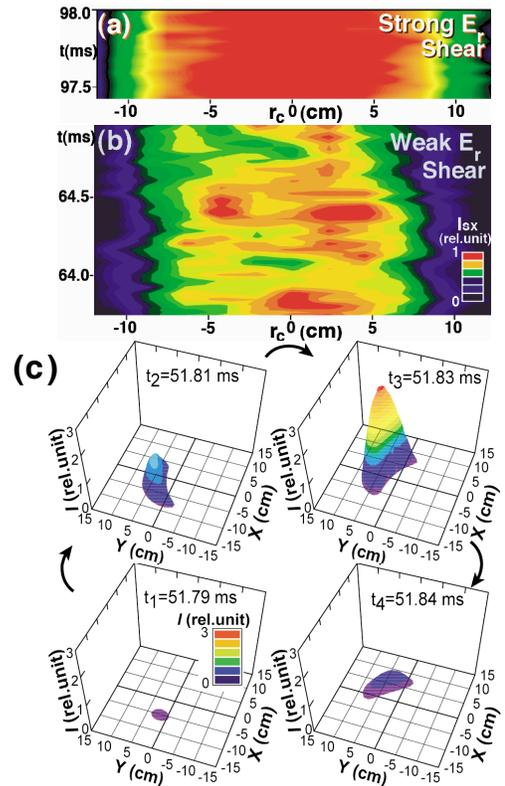
FIG. 4 (color). Contours of central-cell x-ray brightness in the cases with (a) strong and (b) weak  $E_r$  shear formation. “Hot-colored areas” show higher plasma-pressure locations. Vortexlike structures are found in (b). The temporal evolution of a vortex is exemplified in (c) by the use of our developed x-ray tomography systems. ( $I \propto n_e n_i T_e^{2.3}$ .)
