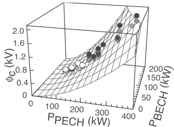
FIG. 1. Three-time advance in  $\phi_c$  including a record of 2.1 kV (filled circles), in comparison to  $\phi_c$  attained 1992–2002 (open circles), extensionally fits well to the scaling surface of  $\phi_c$  with plug ( $P_{\text{PECH}}$ ) and barrier ( $P_{\text{BECH}}$ ) ECH powers (see Refs. [14,15]). Here,  $n_c = 2 \times 10^{18} \text{ m}^{-3}$  is exemplified for a tandem-mirror configuration with  $n_p/n_c = 0.1$  and  $T_i =$  several keV.
