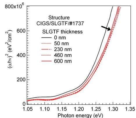
FIG. 6. (Color online) Relation between  $(\alpha hv)^2$  and  $hv$  for CIGS films grown on SLGTF/#1737 substrates.
