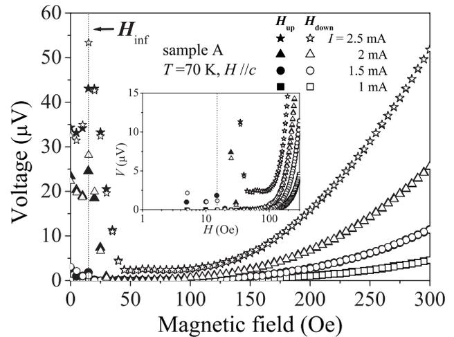
FIG. 5. Field dependence of the voltage at 70 K on sample A for fixed transport currents ( $\parallel a$  axis) above and below the critical current obtained under the self-field. The closed and open symbols represent the ascending and descending branches of the field, respectively. The low-voltage region is enlarged in the inset, where a logarithmic  $H$  scale is used for convenience in displaying the data.
