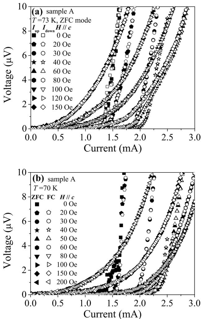
FIG. 2.  $V$ - $I$  characteristics with the configuration of  $I \parallel a$  axis and  $H \parallel c$  axis for sample A. (a)  $V$ - $I$  curves for increasing (closed symbols) and decreasing (open symbols) current at 73 K for the ZFC mode. (b)  $V$ - $I$  curves at 70 K for the ZFC (closed symbols) and FC (open symbols) modes.
