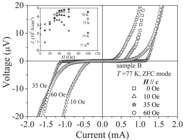
FIG. 4.  $V$ - $I$  characteristics with the configuration of  $I \parallel a$  axis and  $H \parallel c$  axis at 77 K for the ZFC mode for sample B. The inset shows the field dependence of  $J_c$  estimated from the  $V$ - $I$  curves at temperatures in the range 70–77 K.  $H_{\text{peak}}$  varies from 35 to 60 Oe as the temperature is reduced from 77 to 70 K.
