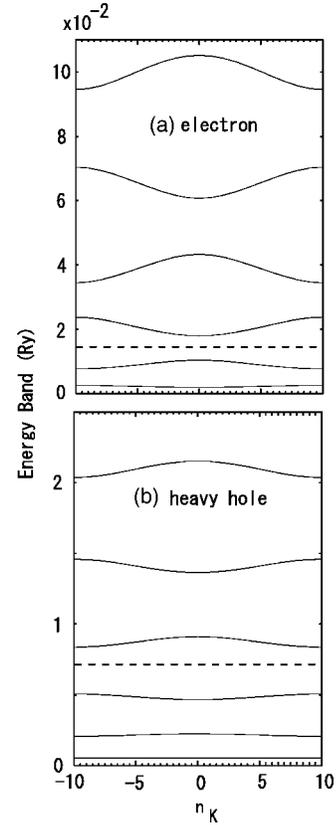
FIG. 1. Energy band structures of the present SLs for (a) the electron and (b) the heavy hole. The horizontal dashed line indicates the height of the confining potential barrier. The abscissae of  $n_K$  are given by  $n_K = N_{site} K d / 2\pi$ , where  $K$  represents the Bloch momentum of the SLs and  $N_{site} = 20$ .
