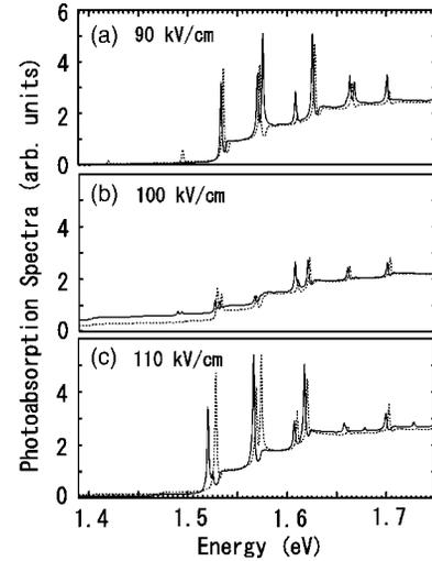
FIG. 11. The calculated FR spectra of the present WSL with  $F$  = (a) 90 kV/cm, (b) 100 kV/cm, and (c) 110 kV/cm as a function of photon energy  $E$ , where the Lorentzian convolution is used with  $\Gamma=2$  meV. The spectra indicated by the solid lines are the same as those in Figs. 9(e)–9(g), while those represented by the dotted lines are the results obtained by the corresponding model calculations. Refer to the text for the details on the calculations of the latter.
