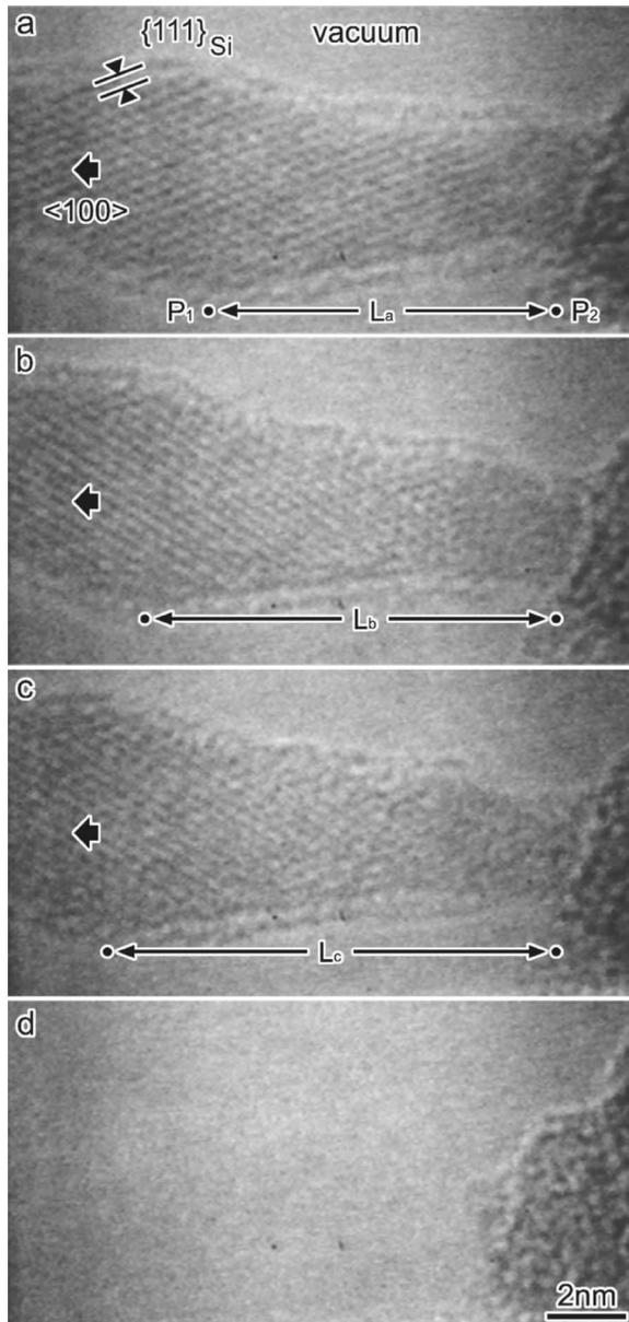
FIG. 2. Time-sequent series of high-resolution images of a tensile deformation process of a single crystalline Si nanowire. The tip of the cantilever (the left-hand side) is retracted towards the left as indicated by the bold arrows.
