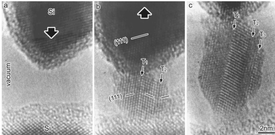
FIG. 1. Time-sequence series of high-resolution images of a nucleation and growth process of a Si nanometer-sized wire. The interval between *a* and *b* is 10 s, and that between *b* and *c* is 11 s. The movement of the tip of the cantilever (upper portion) is indicated by the bold arrows.  $T_i (i=1-3)$  designates twin boundaries.
