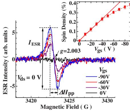
FIG. 2. (Color online) First-derivative field-induced ESR signals obtained for various  $V_{gs}$  values without applying  $V_{ds}$ . The external magnetic field is perpendicular to the substrate. Inset shows the  $V_{gs}$  dependence of the induced spin concentration per thiophene monomer unit. The solid line shows the linear guide to the eye.
