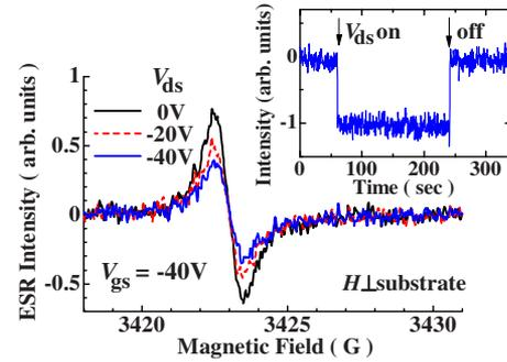
FIG. 3. (Color online) Field-induced ESR signals obtained under the application of  $V_{ds}$  together with  $V_{gs}$  with the external magnetic field perpendicular to the substrate. Inset shows the time response of the field-induced ESR intensity upon the application of  $V_{ds}$ .
