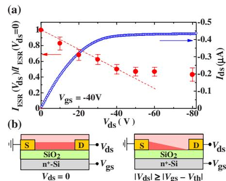
FIG. 4. (Color online) (a)  $V_{ds}$  dependence of the ESR intensity normalized by the value at  $V_{ds} = 0$  under the application of  $V_{gs} = -40$  V (closed circles). The drain current of the FET is also shown for comparison (open circles). The broken line shows the linear guide to the eye. (b) Schematic illustrations of the carrier concentration in the FET channel region for the cases of  $V_{ds} = 0$  and  $|V_{ds}| \geq |V_{gs} - V_{th}|$ .
