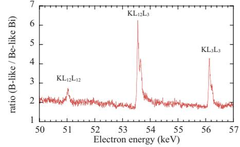
FIG. 1. (Color online) Abundance ratio between B-like and Be-like Bi at equilibrium in the EBIT with an electron-beam current of 80 mA. The enhancements around 51, 53.5, and 56 keV correspond to the *KLL* DR resonances of Be-like Bi.
