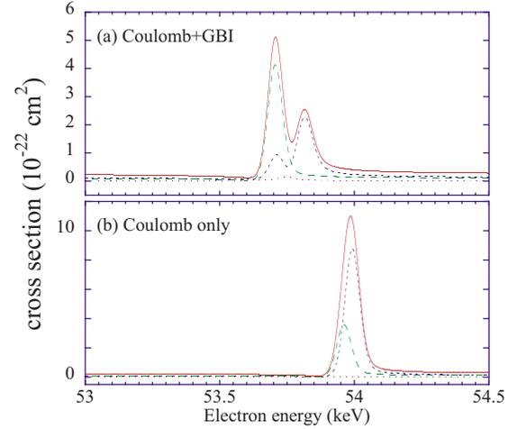
FIG. 3. (Color online) The total recombination cross section for Be-like Bi (solid line) and its partial contributions (long-dashed curve for the intermediate states with  $J=5/2$ ; dashed curve for  $J=3/2$  and dotted curve for  $J=1/2$ ). (a) Results with the generalized Breit interaction [the solid line is the same as Fig. 2(c)]; (b) results considering only the Coulomb interaction. All results are convoluted with the experimental width (60 eV).
