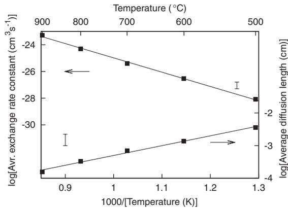
FIG. 4. Temperature dependence of the average exchange rate constant  $k_a$  and the average exchange-free diffusion length  $l$  of an interstitial  $O_2$  molecule [Eq. (7)]. The error bars represent the experimental uncertainties.
