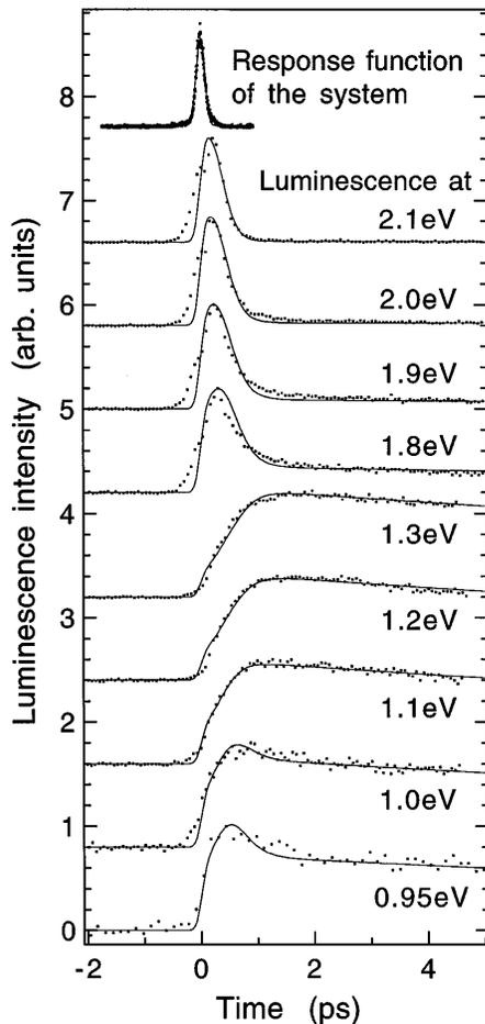
FIG. 3. Time evolution of luminescence from  $-2$  to  $5$  ps. Dots are experimental data. Solid curves show the results of the calculation based on Eq. (2). Intensities are normalized. The zero time delay for each photon energy has been determined by fitting the solid curves to the experimental data. The response function of the system is shown at the top of the figure.
