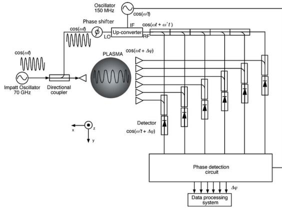
FIG. 1. Schematic of the multichannel microwave interferometer system.
