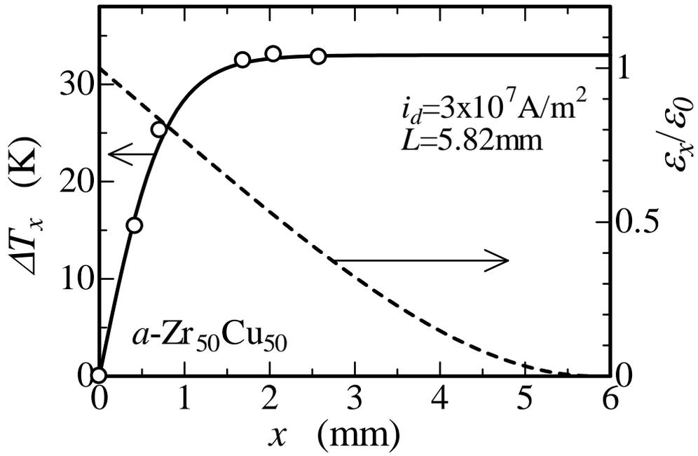
Fig. 4. An example of a change in the temperature along the specimen long axis,  $\Delta T_x$ , during PEC with  $i_d=3.0 \times 10^7 \text{ A/m}^2$  observed for an  $a\text{-Zr}_{50}\text{Cu}_{50}$  specimen ( $\circ$ ). The dashed line denotes the relative change in strain,  $\varepsilon_x/\varepsilon_0$ , estimated from the vibration shape [16].
