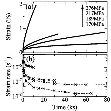
FIG. 3. (a) Examples of the compressive creep curves under various  $\sigma_{ap}$ , 170, 189, 217, and 276 MPa, observed for the type-*H* specimen at 295 K. (b) Differential curves of the creep curves shown in (a).
