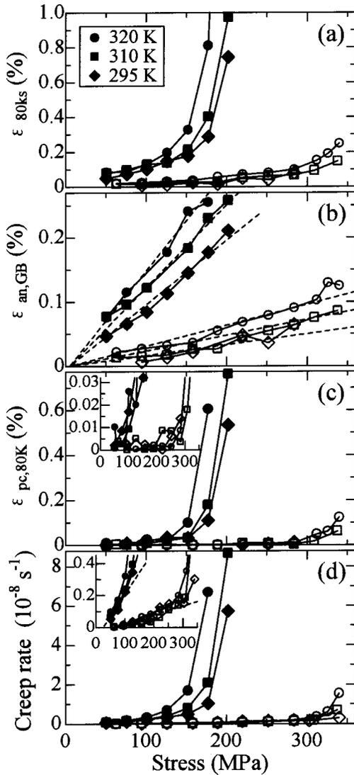
FIG. 2. (a) The  $\varepsilon_{80ks}$  vs  $\sigma_{ap}$  data observed at 295, 310, and 320 K for the type-*H* specimens (filled symbols) and the type-*L* specimens (open symbols). (b)–(d) show the data for  $\varepsilon_{an,GB}$  and  $\varepsilon_{pc}$ , and the creep rate found after a loading time for 80 ks, respectively. See the text for  $\varepsilon_{80ks}$ ,  $\varepsilon_{an,GB}$ ,  $\varepsilon_{pc}$ , and  $\sigma_{ap}$ .
