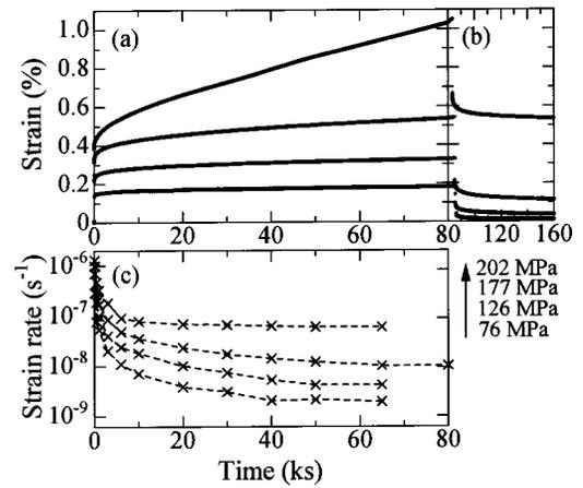
FIG. 1. (a) Examples of the tensile creep curves measured under  $\sigma_{ap}$  of 76, 126, 177, and 202 MPa. (b) Elastic aftereffect curves after unloading. These measurements were sequentially made at 295 K for the type- $H$  specimen. (c) Differential curves of the creep curves shown in (a).
