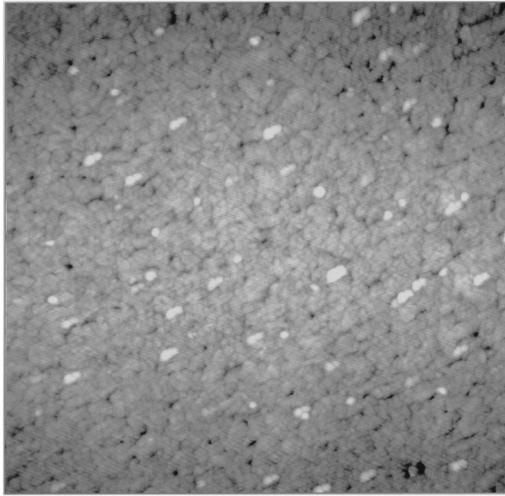
FIG. 6. An example of the STM images observed for the type- $L$  specimen before the creep test. The scanning area is  $1000 \times 1000 \text{ nm}^2$ , and the black to white contrast measures a change in height as 5 nm.
