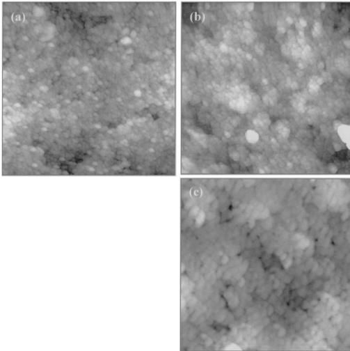
FIG. 10. Examples of the STM images observed after the creep tests in region III, which were made by the micro-Vicker's hardness, (a) for the type-*H* specimen, and (b) and (c) for the type-*L* specimen. The scanning area and the black to white height are  $1000 \times 1000 \text{ nm}^2$  and 5 nm for (a),  $1000 \times 1000 \text{ nm}^2$  and 7 nm for (b), and  $500 \times 500 \text{ nm}^2$  and 7 nm for (c), respectively. See the text for testing conditions.
