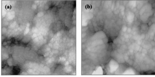
FIG. 9. Similar to Figs. 8(a) and 8(c) but here the STM images observed for the type-*H* specimen after the tensile creep test at 295 K with the increased  $\sigma_{ap}$  of 200 MPa in region II are shown, where the plastic creep deformation attained was 10%. The scanning area and the black to white height are  $1000 \times 1000 \text{ nm}^2$  and 25 nm for (a) and  $500 \times 500 \text{ nm}^2$  and 12 nm for (b), respectively.
