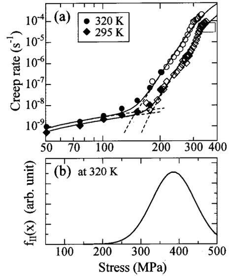
FIG. 12. (a) The best fitting of Eqs. (3) and (10) (the solid curves) to the creep rate vs stress data at 295 K and those at 320 K observed for the type- $H$  specimen. (b) The Gaussian distribution function  $f_{II}(x)$  found for the creep rate data at 320 K shown in (a).
