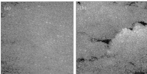
FIG. 7. Examples of the STM images observed for the type- $H$  specimen after plastic creep deformation by 0.3% at 295 K under 100 MPa in region I. (a) Most of the specimen surface, (b) A mesoscopic scale GB slip observed here and there, but the areal density is very low. The scanning area is  $1000 \times 1000 \text{ nm}^2$ , and the black to white height is 6 nm for (a) and 11 nm for (b), respectively.
