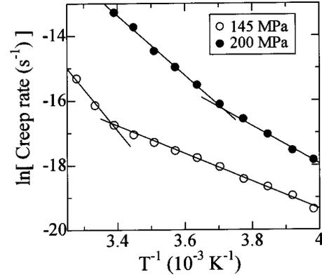
FIG. 5. Examples of the Arrhenius plot for  $\varepsilon'$  in regions I and II, where the  $\varepsilon'$  data were observed in the tensile creep tests at 145 and 200 MPa for the type-*H* specimen.
