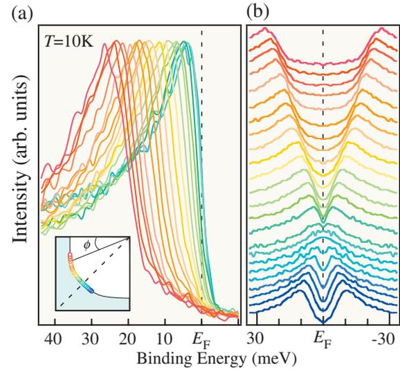
FIG. 2. (Color) (a) ARPES spectra for pristine Bi2212 measured at 10 K at several  $k_F$  points of the antibonding band. Location of  $k_F$  points is indicated by differently colored circles in the Brillouin zone (inset). (b) Symmetrized ARPES spectra in (a).
