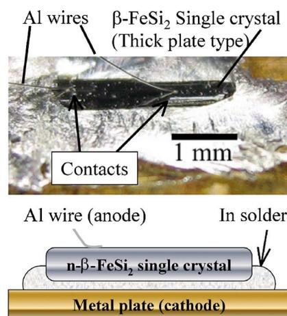
FIG. 1. (Color online) Typical photograph of Al/ $\beta$ -FeSi<sub>2</sub> and a schematic cross section of the device. This device has two Al wires connected to the front surface of  $\beta$ -FeSi<sub>2</sub>. The back surface contact was formed with In solder.
