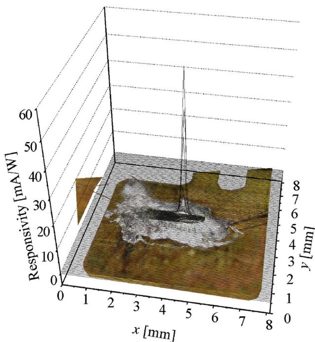
FIG. 3. (Color online) Mapping of photoresponsivity under laser illumination. The wavelength and the output power of the laser were 1.31  $\mu$ m and 1.0 mW, respectively. The spot size was approximately 50  $\mu$ m.
