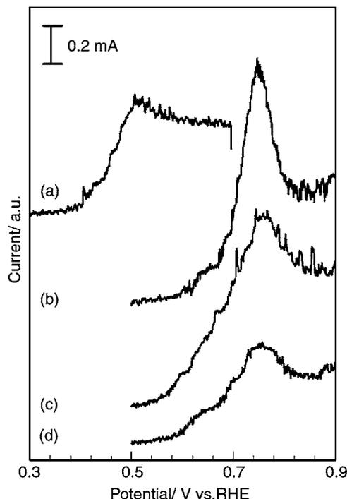
**Figure 4.** CO stripping voltammetry after keeping the potential at 0.1 V RHE for 10 min in hydrogen gas containing 1% CO: (a) Pt-Ru/C, (b) Pt-[Lu<sub>2</sub>Cu<sub>4</sub>(f-saaep)<sub>4</sub>]/C, (c) Pt-[Pr<sub>2</sub>Cu<sub>4</sub>(f-saaep)<sub>4</sub>]/C, and (d) Pt-[Gd<sub>2</sub>Cu<sub>4</sub>(f-saaep)<sub>4</sub>]/C.
