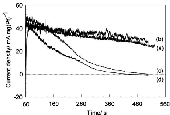
**Figure 3.** Time variation of HOR current density on RDE with various catalysts measured in 0.1 mol dm<sup>-3</sup> HClO<sub>4</sub>, after keeping the potential for 60 s at 0.8 V vs RHE and then at 0.1 V vs RHE for 600 s: (a) Pt-Ru/C, (b) Pt-[Lu<sub>2</sub>Cu<sub>4</sub>(f-saaep)<sub>4</sub>]/C, (c) Pt-[Pr<sub>2</sub>Cu<sub>4</sub>(f-saaep)<sub>4</sub>]/C, and (d) Pt-[Gd<sub>2</sub>Cu<sub>4</sub>(f-saaep)<sub>4</sub>]/C.
