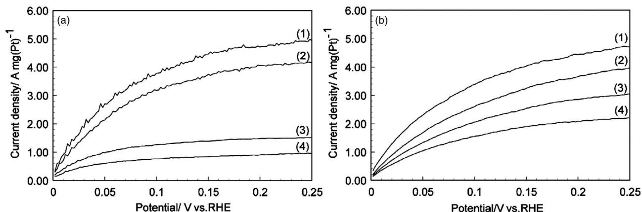
**Figure 5.** Current–potential curves under various amounts of CO for (a) Pt–Ru/C and (b) Pt–[Lu<sub>2</sub>Cu<sub>4</sub>(f<sub>s</sub>aaep)<sub>4</sub>]/C: (1) pure H<sub>2</sub>, (2) 10 ppm CO/H<sub>2</sub>, (3) 50 ppm CO/H<sub>2</sub>, and (4) 100 ppm CO/H<sub>2</sub>.
