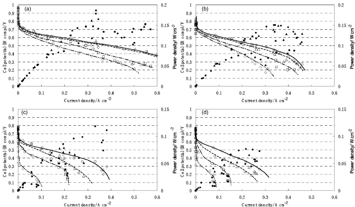
**Figure 6.** Polarization curves and power density–current density curves of (a) Pt–Ru/C, (b) Pt–[Lu<sub>2</sub>Cu<sub>4</sub>(f<sub>s</sub>aaep)<sub>4</sub>]/C, (c) Pt–[Pr<sub>2</sub>Cu<sub>4</sub>(f<sub>s</sub>aaep)<sub>4</sub>]/C, and (d) Pt–[Gd<sub>2</sub>Cu<sub>4</sub>(f<sub>s</sub>aaep)<sub>4</sub>]/C measured with a PEFC single cell. Anode gas: H<sub>2</sub>(○), H<sub>2</sub> + 10 ppm CO (△), H<sub>2</sub> + 50 ppm CO(□), and H<sub>2</sub> + 100 ppm CO(◇).
