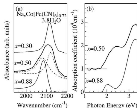
FIG. 1. (a) Infrared absorption spectra of  $\text{Na}_x\text{Co}[\text{Fe}(\text{CN})_6]_{0.72}\cdot 3.8\text{H}_2\text{O}$ . Broken curves are the result of the least-square-fitting with two Lorentz functions. (b) Visible absorption spectra of  $\text{Na}_x\text{Co}[\text{Fe}(\text{CN})_6]_{0.72}\cdot 3.8\text{H}_2\text{O}$ .
