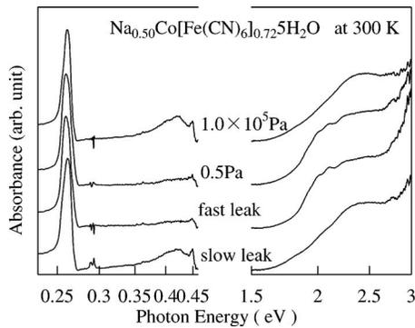
FIG. 2. Infrared and visible absorption spectra of  $\text{Na}_{0.50}\text{Co}[\text{Fe}(\text{CN})_6]_{0.723}\cdot 3.8\text{H}_2\text{O}$  under various pressure conditions. A downward arrow indicates the OH stretching band. A broken curve in the left panel is the differential spectra between the ambient pressure spectrum and the vacuum spectrum.
