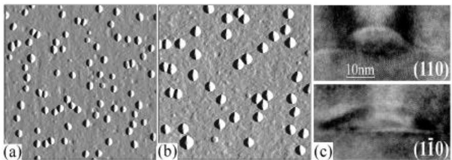
**Figure 1.** AFM images ( $1\mu m \times 1\mu m$ ) of 4ML InP islands grown on 4ML GaP/GaInP at (a)  $550^\circ C$  and (b)  $600^\circ C$ , (c) TEM images of  $550^\circ C$  grown InP dots in the (110) and ( $\bar{1}10$ ) cross-sections.
