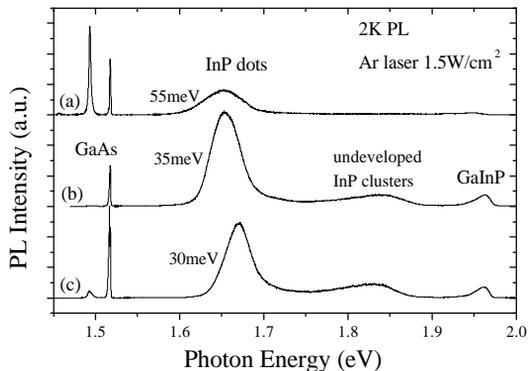
**Figure 3.** 2K PL of InP/GaInP dots (a) with no GaP spacer, (b) with a 4ML GaP spacer below the InP dots, (c) with a 4ML GaP spacer below and a 2ML GaP spacer above the InP dots.
