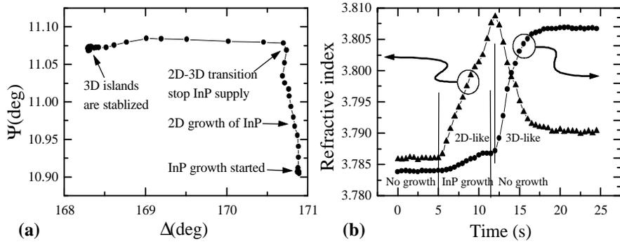
**Figure 2.** The  $\Delta$ - $\Psi$  trajectory and change of  $n$ ,  $k$  (b) during the growth of InP dots showing the 2D-3D transition by fast-nulling ellipsometer. The sampling time is 25ms and data interval is 0.5s.
