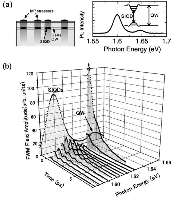
FIG. 1. (a) The structure of the strain-induced GaAs quantum dots and PL spectrum at 2 K. The shades schematically represent strain fields due to InP stressors. (b) FWM signals excited by various photon energies at 20 K. For this measurement, the spectral width of the laser was reduced to 15 meV.
