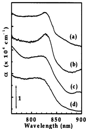
FIG. 1. Absorption spectra of Be-doped ( $7.8 \times 10^{17} \text{ cm}^{-3}$ ) GaAs/AlAs MQWs grown at (a) 600, (b) 360, and (c) 310 °C. Also, shown a spectrum of Be-doped ( $2 \times 10^{19} \text{ cm}^{-3}$ ) MQW grown at 280 °C in (d).
