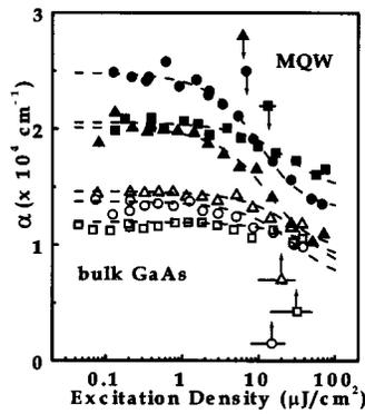
FIG. 3. Excitation density dependence of the apparent optical absorption coefficient  $\alpha$  in Be-doped ( $7.8 \times 10^{17} \text{ cm}^{-3}$ ) bulk GaAs (open symbols) and GaAs/AlAs MQWs (closed symbols) grown at 600 ( $\Delta$ ), 360 ( $\bullet$ ), and 310 ( $\square$ )  $^{\circ}\text{C}$ . Dashed curves are fits to the data. Arrows show the saturation density  $F_{\text{sat}}$  for each sample, and error ranges are indicated by bars.
