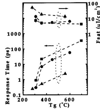
FIG. 4. Response time  $\tau$  and saturation density  $F_{\text{sat}}$  of GaAs/AlAs MQWs plotted against growth temperature  $T_g$ : undoped ( $\blacksquare$ ),  $[\text{Be}] = 7.8 \times 10^{17} \text{ cm}^{-3}$  ( $\bullet$ ), and  $[\text{Be}] = 2 \times 10^{19} \text{ cm}^{-3}$  ( $\blacktriangle$ ).
