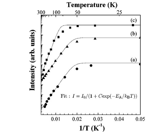
FIG. 3. The temperature dependence of the integrated PL intensity of samples (a)–(c). The solid lines show the result of fitting to the equation  $I = I_0 / [1 + C \exp(-E_A/k_B T)]$ . From the fitting, we obtained the activation energy  $E_A = 59$  meV for samples (a), (b) and  $E_A = 110$  meV for sample (c).
