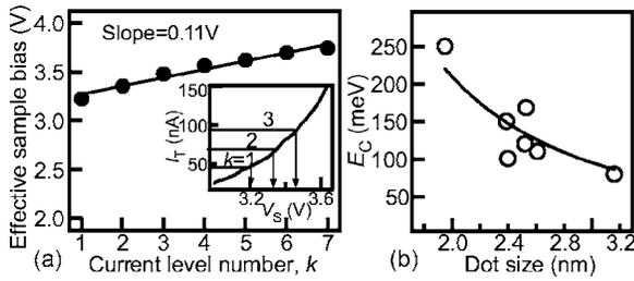
FIG. 2. (a)  $V_S^e$ 's estimated from  $I_T$ - $V_S$  curve of the 2.6 nm OD in the inset were aligned with a slope of  $\sim 0.11$  V for the discrete tunneling current levels denoted as  $k(=1, 2, \dots)$ . (b) The dot size dependence of  $E_C$  in QDs measured at  $V_S = +3$  V. The fitting curve is determined using Eq. (1) with  $a \sim 1.3$ .
