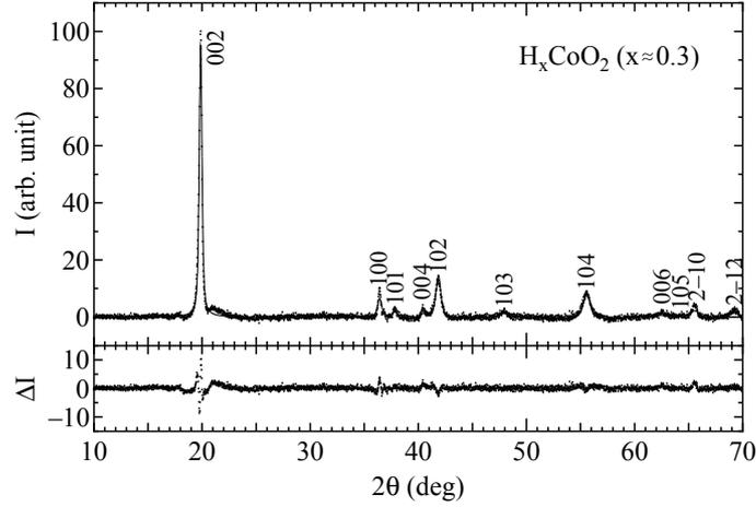
**Figure 1.** The x-ray powder diffraction pattern with Cu  $K\alpha$  radiation at 293 K for the specimens derived through chemical extraction of Na from the nominal compound  $\text{Na}_{0.3}\text{CoO}_2$  using  $\text{H}_2\text{SO}_4$ . The result in terms of Rietveld refinement is indicated by a full curve in the top panel and the difference between the observed and calculated intensities is plotted in the bottom panel.
