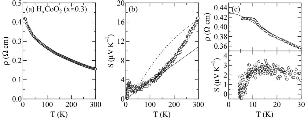
**Figure 3.** The temperature dependences of (a) the electrical resistivity and (b) the thermoelectric power for  $H_x\text{CoO}_2$  ( $x \approx 0.3$ ), and (c) their low-temperature parts. The full curves in (a) and (c) denote a fit to equation (1), and the full line and dotted curve in (b) are fits to equations (4) and (5), respectively, with parameters given in the text
