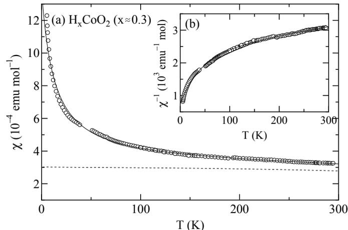
**Figure 4.** The temperature dependences of (a) the magnetic susceptibility and (b) its inverse for  $H_x\text{CoO}_2$  ( $x \approx 0.3$ ). The full curves in (a) and (b) denote fits to equation (8) with parameters given in the text, and the dotted curve in (a) indicates a contribution from the first and second terms in that equation.
