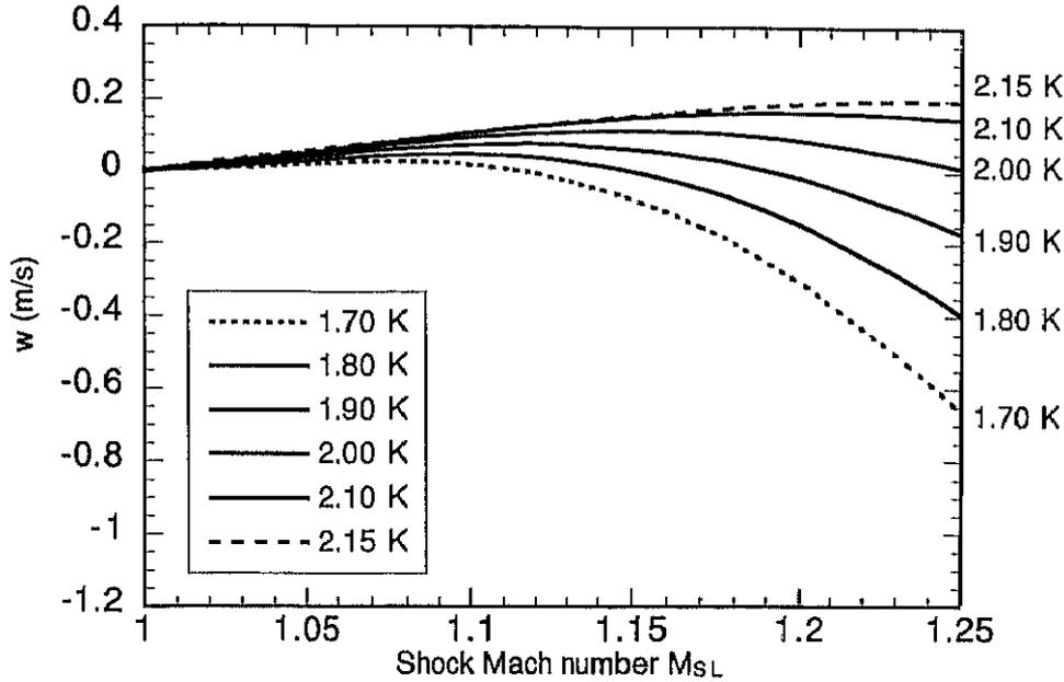
Figure 5.29: Counterflow velocity  $w$  behind a compression shock wave *vs.* shock Mach number  $M_{SL}$ .
