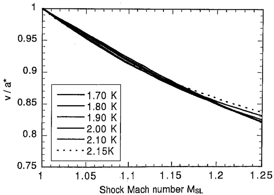
Figure 5.26: Normalized flow velocity  $v/a^*$  behind a compression shock wave *vs.* shock Mach number  $M_{SL}$ .
