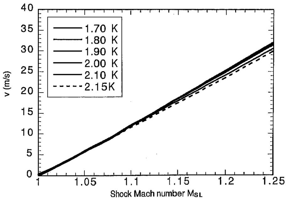
Figure 5.28: Flow velocity  $v$  behind a compression shock wave *vs.* shock Mach number  $M_{SL}$ .
