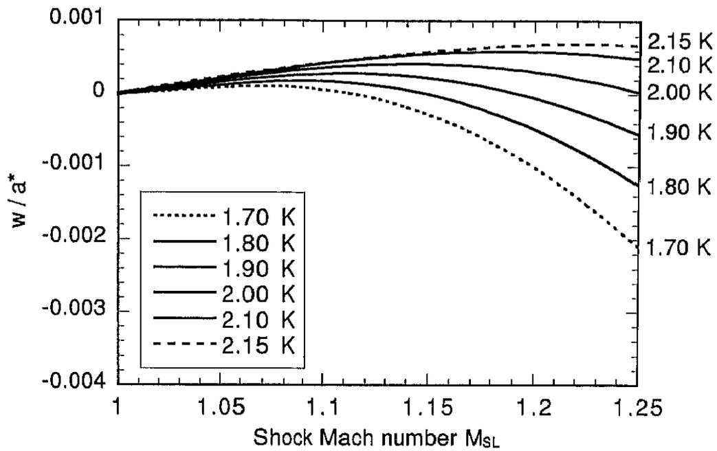
Figure 5.27: Normalized counterflow velocity  $w/a^*$  behind a compression shock wave *vs.* shock Mach number  $M_{SL}$ .
