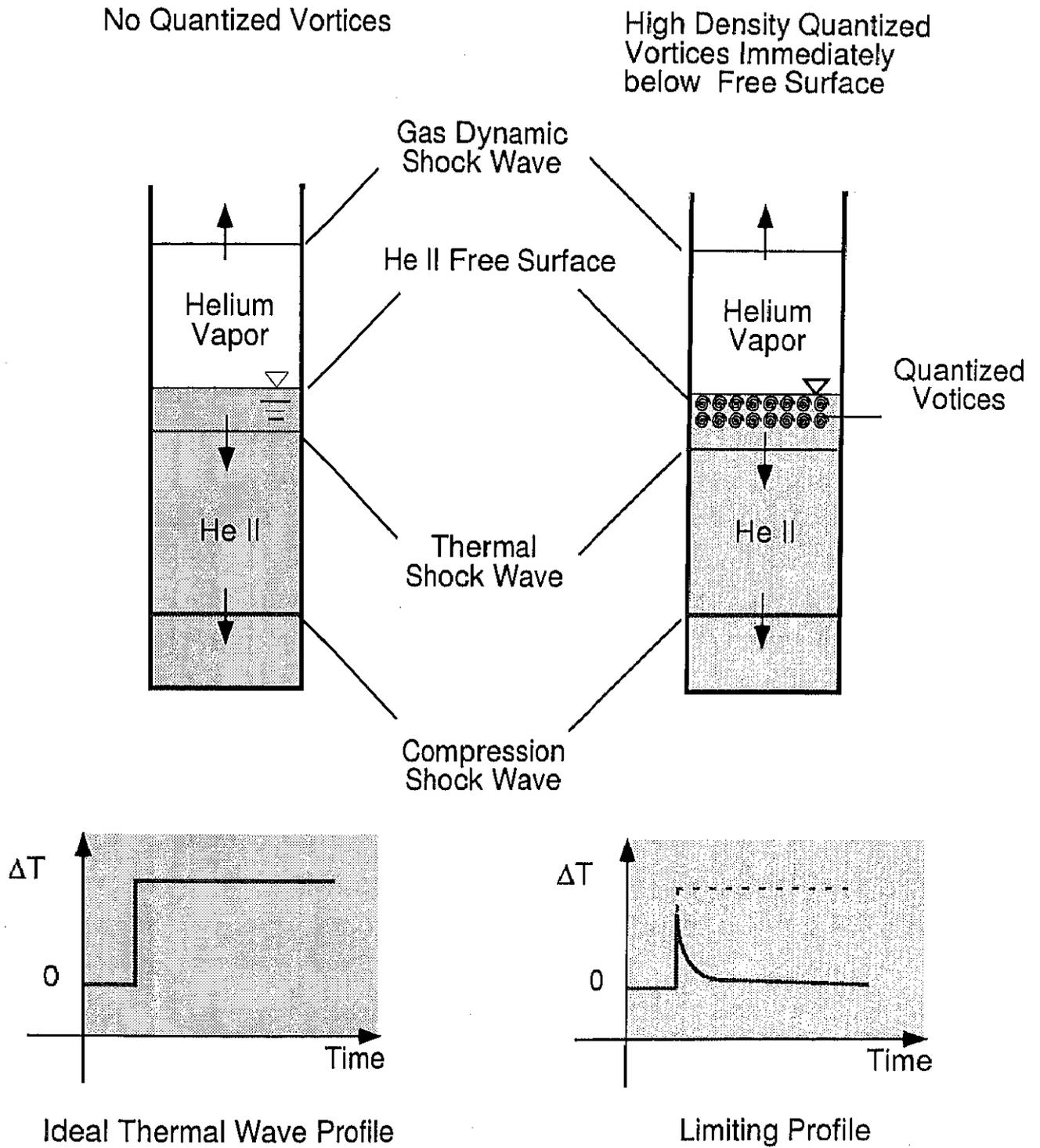
Figure 5.34: Schematic illustration of appearance of limiting profile.
