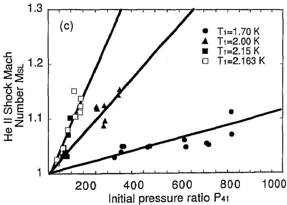
Figure 5.10: Shock wave performance of superfluid shock tube facility.  $p_{41}$  vs.  $\Delta p$  in *HeII*;  $\Delta p$  = pressure jump of transmitted compression shock wave in *HeII*.
