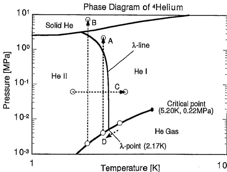
Figure 5.38: Schematic illustration of various methods due to phase transitions. A:  $\lambda$ -phase transition by shock compression. B: *HeII*-solid helium phase transition by shock compression. C:  $\lambda$ -phase transition by heating. D:  $\lambda$ -phase transition by cooling.
