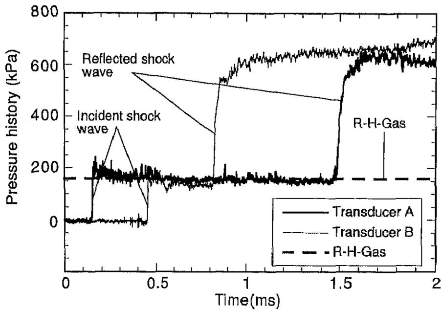
Figure 5.1: Pressure history of typical shock wave. (driver gas; helium, driven gas; nitrogen)  $p_4 = 425.5 \text{ kPa}$ ,  $p_1 = 53.50 \text{ kPa}$ ,  $p_{41} = 7.95$ ,  $U_{SV} = 664 \text{ m/s}$ ,  $M_{SV} = 1.90$ , Both gases at  $293 \text{ K}$
