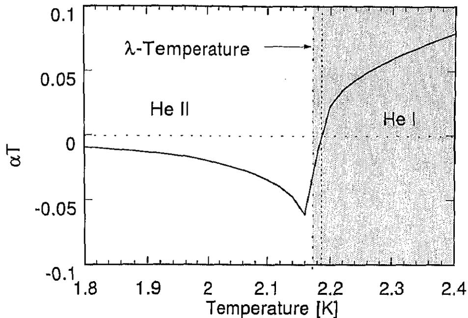
Figure 5.42: Thermal expansion coefficient of liquid helium,  $\alpha$ , along saturated vapor pressure.  $\alpha$ : Thermal expansion coefficient.
