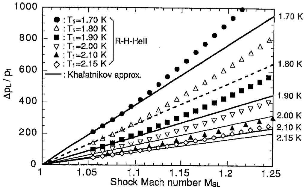
Figure 5.22: Pressure jump  $\Delta p/p_1$  vs. shock Mach number  $M_{SL}$ .
