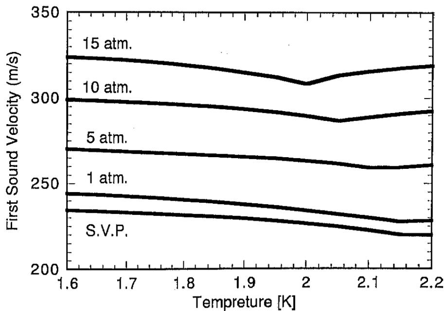
Figure 5.15: Dependence of first-sound velocity on temperature and pressure. *S.V.P.* is the saturated vapor pressure.
