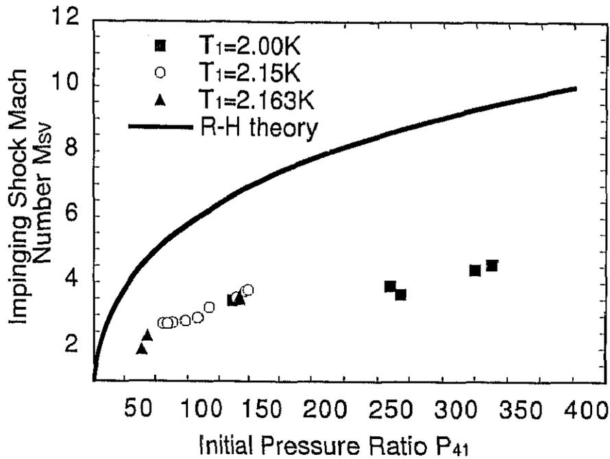
Figure 5.7: Shock wave performance of superfluid shock tube facility.  $p_{41}$  vs.  $M_{SV}$ ;  $M_{SV}$  = impinging shock Mach number in the vapor.  $p_{41} = p_4/p_1$ ,  $p_4$  = pressure of high-pressure helium in the driver section.  $p_1$  = initial pressure of saturated helium vapor in the driven section.
