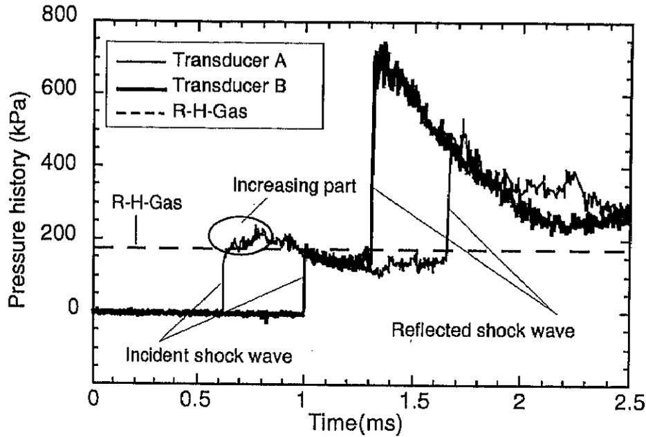
Figure 5.3: Pressure history in the case of saturated nitrogen vapor 77 K in the low-pressure tube section. (driver gas; helium, driven gas; nitrogen)  $p_4 = 425.5 \text{ kPa}$ ,  $p_1 = 19.50 \text{ kPa}$ ,  $p_{41} = 21.81$ ,  $U_{SL} = 529 \text{ m/s}$ ,  $M_{SV} = 3.02$
