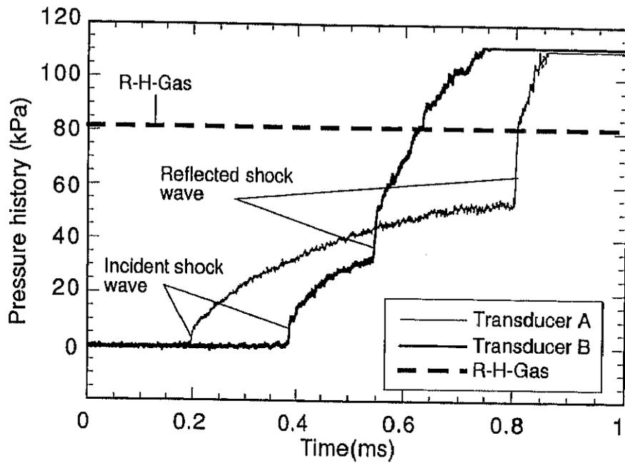
Figure 5.4: Pressure history in the case of helium gas. (driver gas; helium, driven gas; helium)  $p_4 = 425.5 \text{ kPa}$ ,  $p_1 = 53.5 \text{ kPa}$ ,  $p_{41} = 7.95$ ,  $U_{SL} = 1060 \text{ m/s}$ ,  $M_{SV} = 1.05$ , Both gases at  $293 \text{ K}$
