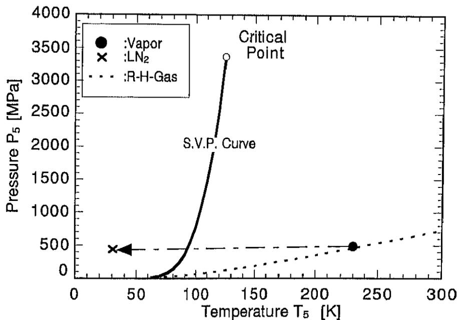
Figure 5.21: Thermodynamic state near liquid nitrogen free surface. ●:behind reflected vapor shock. ×:behind transmitted shock in *LN<sub>2</sub>*. The dotted line is *R-H-Gas* relation between  $T_5$  and  $p_5$  for 65 K.
