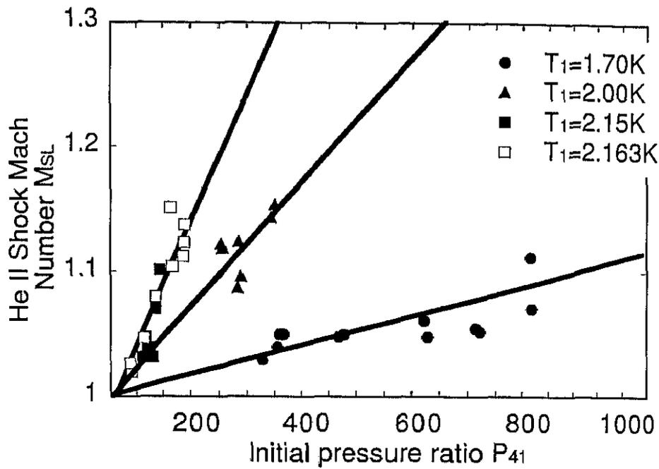
Figure 5.9: Shock wave performance of superfluid shock tube facility.  $p_{41}$  vs.  $M_{SL}$ ;  $M_{SL}$  = Shock Mach number of transmitted compression shock wave in *HeII*.
