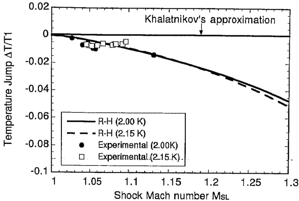
Figure 5.17: Variation of the temperature jump  $\Delta T$  at the wave front of the transmitted compression shock wave with the shock Mach number  $M_{SL}$ . The solid and dotted lines are the numerical calculation results based on  $R-H-HeII$  relation for  $T_1 = 2.00 K$  and  $2.15 K$ , and Khalatnikov's approximation result, that is  $\Delta T = 0$ .
