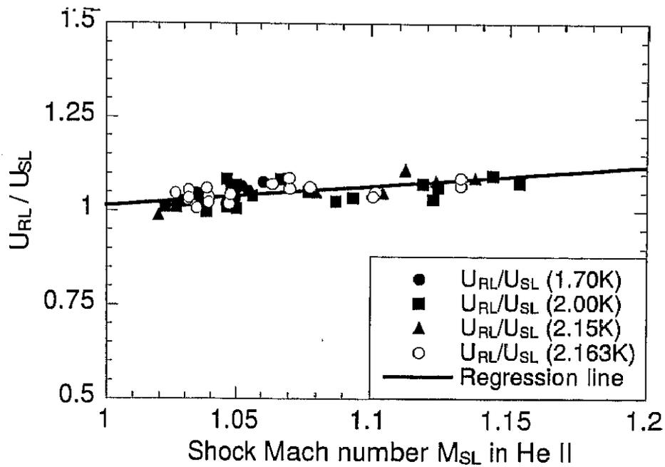
Figure 5.14:  $U_{RL}/U_{SL}$  versus Transmitted shock Mach number  $M_{SL}$ .  $U_{SL}$  is the incident shock speed and  $U_{RL}$  is the reflected shock speed.
