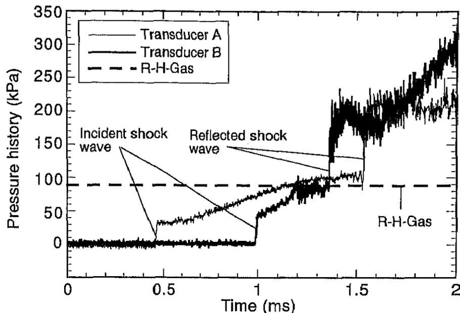
Figure 5.6: Pressure history in the case of saturated helium vapor at 2K in the low-pressure tube section. (driver gas; helium, driven gas; helium)  $p_4 = 567.4 \text{ kPa}$ ,  $p_1 = 2.06 \text{ kPa}$ ,  $p_{41} = 274.6$ ,  $U_{SL} = 373 \text{ m/s}$ ,  $M_{SV} = 4.66$
