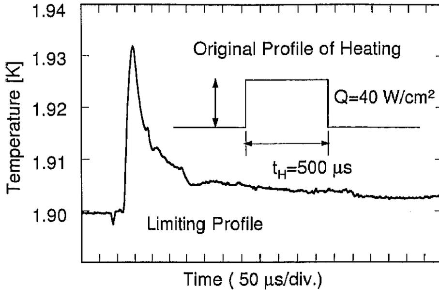
Figure 5.33: Temperature variation caused by stepwise heating in *HeII*; a limiting profile.  $T_1 = 1.90\text{ K}$ ,  $Q = 40\text{ W/cm}^2$ , Heating time  $t_H = 500\text{ }\mu\text{s}$   $Q$ : Input heat flux
