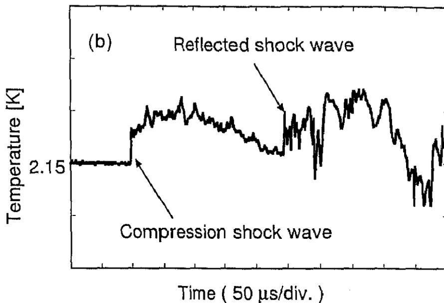
Figure 5.40: Transient record of the  $\lambda$ -transition from *HeII* to *HeI* induced by shock compression.  $T_1 = 2.15$  K.
