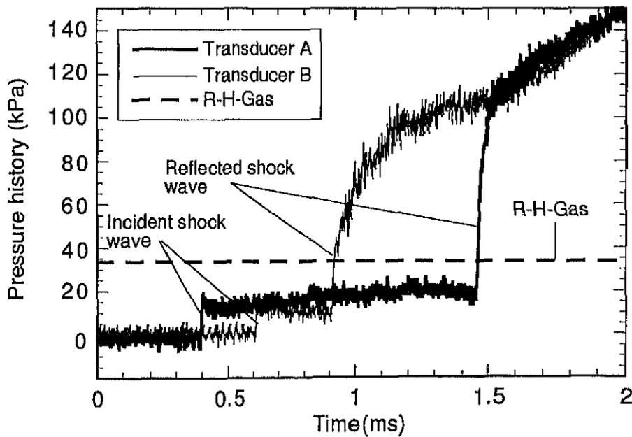
Figure 5.2: Pressure history of typical shock wave. (driver gas; helium, driven gas; nitrogen)  $p_4 = 425.5 \text{ kPa}$ ,  $p_1 = 1.50 \text{ kPa}$ ,  $p_{41} = 278.14$ ,  $U_{SV} = 934 \text{ m/s}$ ,  $M_{SV} = 2.67$ , Both gases at  $293 \text{ K}$
