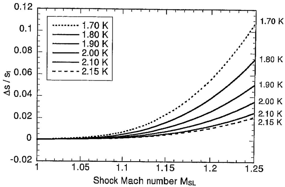
Figure 5.30: Entropy jump  $\Delta s/s_1$  vs. shock Mach number  $M_{SL}$ .
