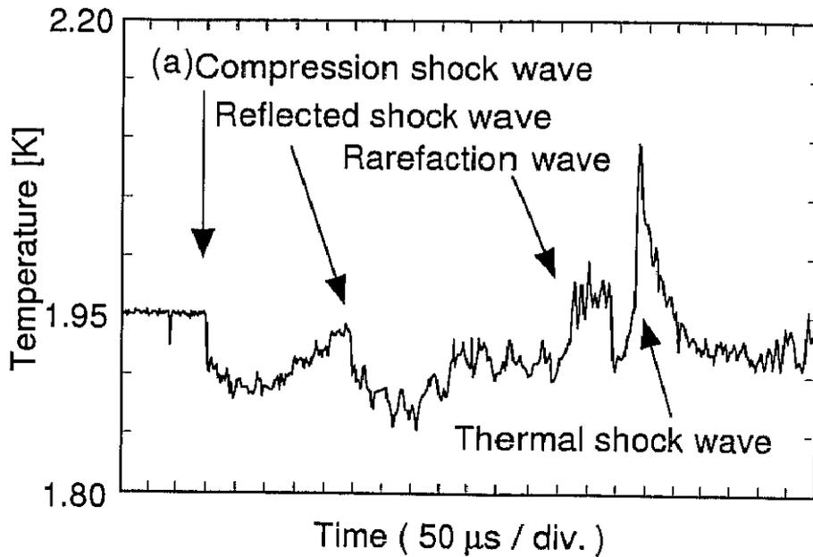
Figure 5.39: Transient record of the *HeII* compression results without  $\lambda$ -phase transition.  $T_1 = 1.95$  K.
