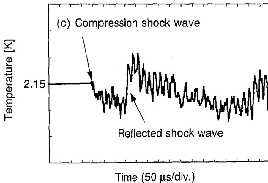
Figure 5.41: A special case with  $\lambda$ -transition.; from *HeII* to *HeI*, resulting from shock compression by reflected compression shock wave from the shock tube bottom.  $T_1 = 2.15$  K.
