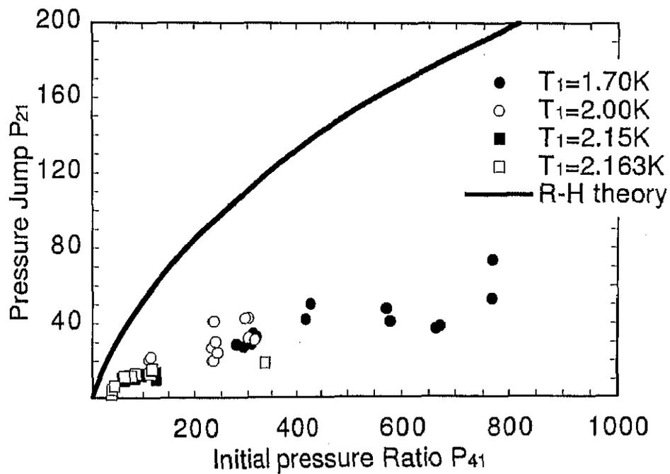
Figure 5.8: Shock wave performance of superfluid shock tube facility.  $p_{41}$  vs. pressure jump  $p_{21}$ ;  $p_{21} = p_2/p_1$ ,  $p_2$  = wave front pressure of impinging shock wave in the vapor.
