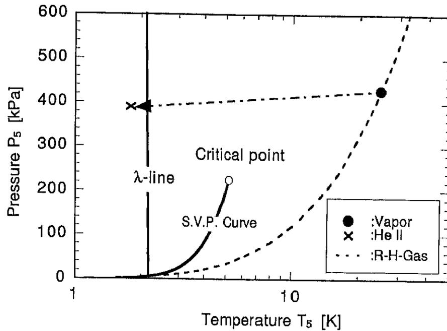
Figure 5.20: Thermodynamic state near *HeII* free surface. ●:behind reflected vapor shock . ×:behind transmitted shock in *HeII*. The dotted line is *R-H-Gas* relation between  $T_5$  and  $p_5$  for 2.15 K.
