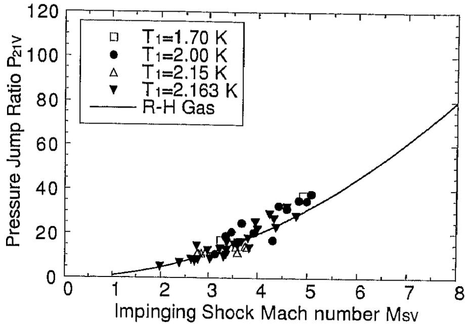
Figure 5.11: Impinging shock wave condition in the helium vapor.  $p_{21}$  vs.  $M_{sv}$  Solid line is the Rankine-Hugoniot relation (*R-H-Gas*).
