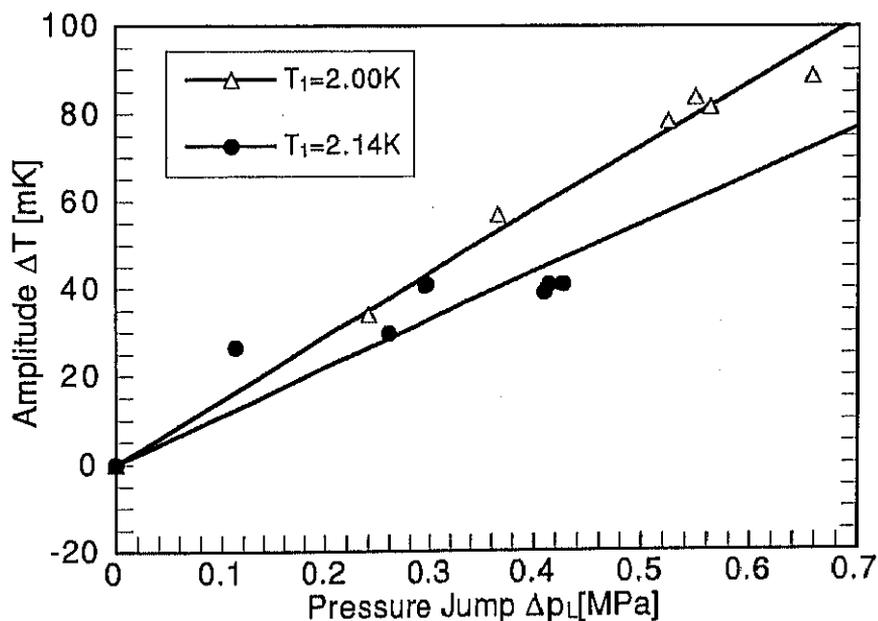
Figure 5.35: The amplitude of thermal shock wave  $\Delta T$  as a function of pressure jump of transmitted compression shock wave  $\Delta p_L$ .
