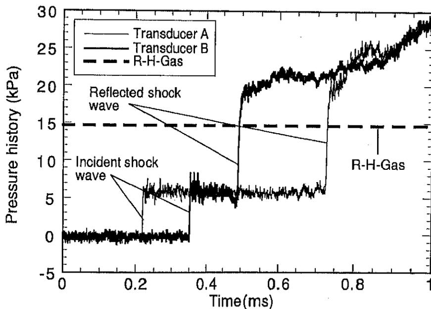
Figure 5.5: Pressure history in the case of helium gas. (driver gas; helium, driven gas; helium)  $p_4 = 425.5 \text{ kPa}$ ,  $p_1 = 2.66 \text{ kPa}$ ,  $p_{41} = 159.6$ ,  $U_{SL} = 1520 \text{ m/s}$ ,  $M_{SV} = 1.51$ , Both gases at  $293 \text{ K}$
