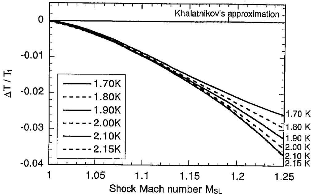
Figure 5.23: Temperature jump  $\Delta T/T_1$  vs. shock Mach number  $M_{SL}$ .
