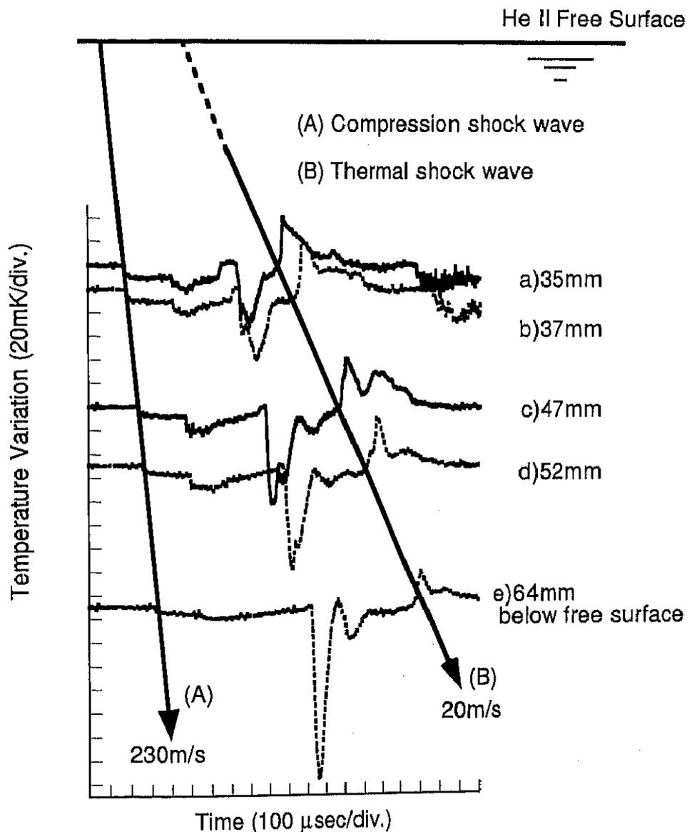
Figure 5.36: Time variations of the temperature resulting from compression shock waves and a thermal shock wave measured at five locations; (a) 35 mm below free surface, (b) 37 mm, (c) 47 mm, (d) 52 mm, (e) 64 mm.
