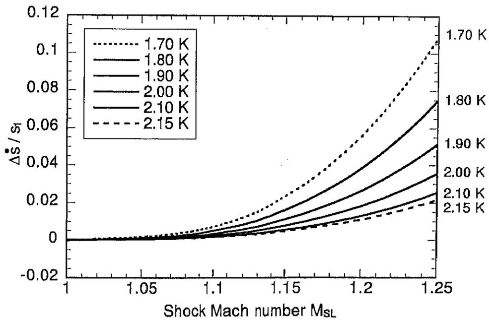
Figure 5.31: Entropy flux jump  $\Delta \dot{s}/s_1$  vs. shock Mach number  $M_{SL}$ .
