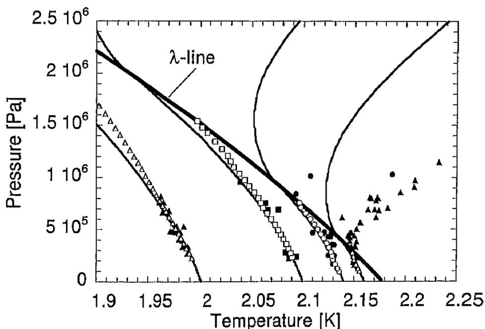
Figure 5.44: The temperature and pressure at the wave front of compression shock wave in *HeII* plotted for four initial temperatures of *HeII*. Solid lines are adiabatic curves (isentropic lines). Open circle are shock adiabatics. Closed circle are experimental data points.
