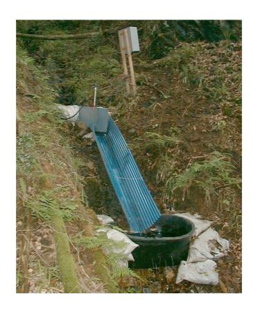
Photo 6: A bedload trap and a flume at C1L site
