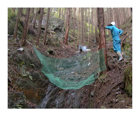
Photo 8: A bedload trap and a flume at C3L site
