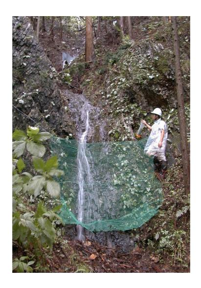
Photo 7: A bedload trap and a flume at C3U site Photograph was taken during a storm runoff on 9 July 2000.
