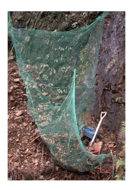
Photo 10: The bedload trap torn by debris at C3U site Photograph was taken on 1 September 2001.
