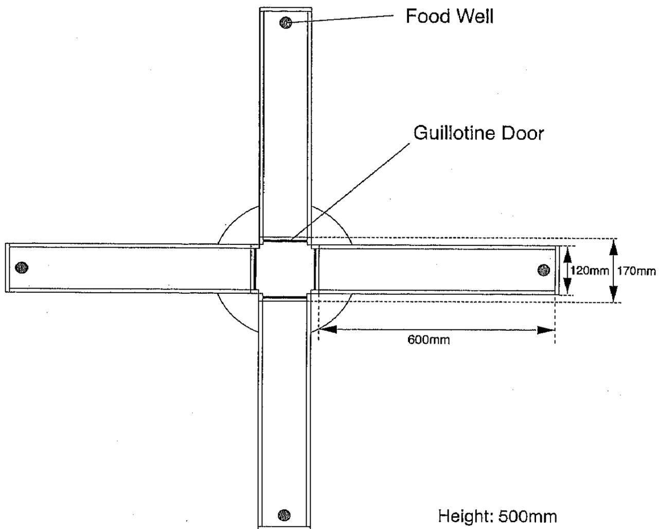
Fig. 19. Illustration of the elevated plus maze.
