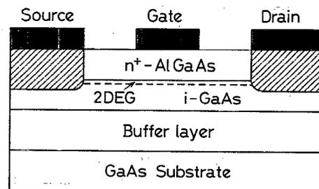
FIG. 7. Cross section of a HEMT structure.
