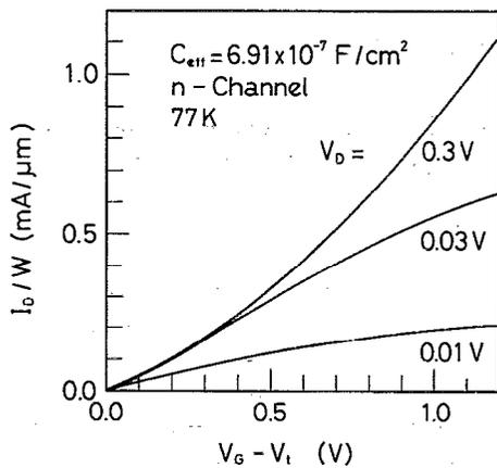
FIG. 5. Calculated examples of  $I$ - $V$  characteristics of an  $n$ MOSFET on (100) plane.  $C_{\text{eff}}$  corresponds to effective 5 nm oxide thickness: (a) channel current per unit width vs drain voltage, parameter is the gate voltage; (b) channel current per unit width versus gate voltage, parameter is the drain voltage.
