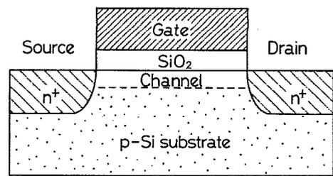
FIG. 1. The cross section of a bulk-type  $n$ MOSFET with an intrinsic channel region.
