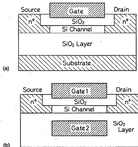
FIG. 2. The cross section of the ultrathin SOI  $n$ MOSFET where the channel region is made of intrinsic silicon: (a) the single gate MOSFET, (b) the dual gate MOSFET.
