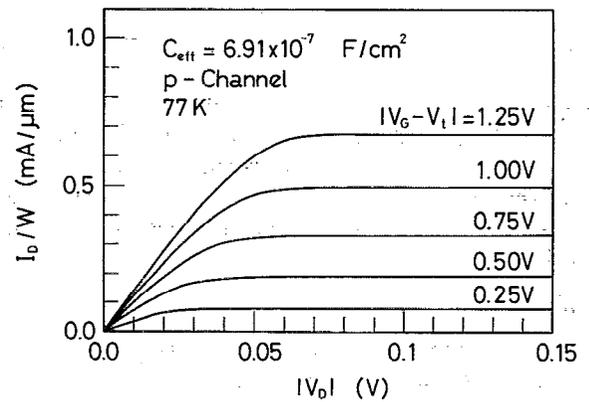
FIG. 6.  $I$ - $V$  characteristics of a  $p$ -channel MOSFET. Channel current per unit width vs drain voltage with the gate voltage as the parameter.  $C_{\text{eff}}$  corresponds to effective 5 nm oxide thickness.  $M_v=1$  is assumed.
