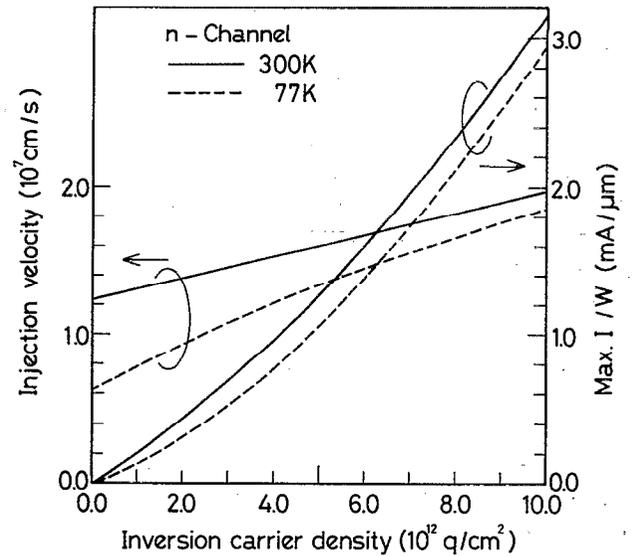
FIG. 8. Saturation current per unit width and the injection velocity of a  $n$ MOSFET on (100) plane as functions of inversion carrier density. The current value gives the maximum limit of the MOSFET current.
