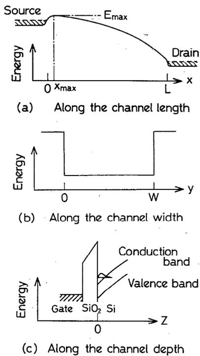
FIG. 3. Schematic distribution of electronic potential energy in a MOSFET structure: (a) the potential distribution along the channel length; (b) the potential distribution along the MOSFET width; (c) the electronic energy distribution along the channel thickness direction.
