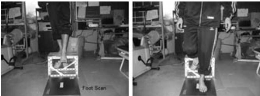
Figure2 Landing movement from the 30cm high box to "Foot Scan".
