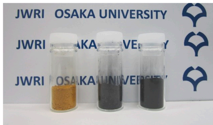
Figure 1. Photographs of (left) \alpha -FeOOH powder used as a precursor; (center) the product prepared by reducing \alpha -FeOOH in the mixed solvent with 9 vol. % water concentration at 200 °C for 24 h; (right) the product prepared by reducing \alpha -FeOOH with 12 vol. % water concentration at 200 °C for 48 h.
