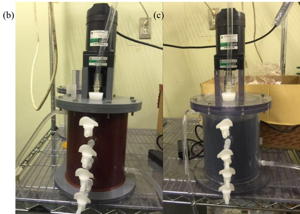
Figure 4-1 The structure figures of CSTR: (a) schematic figure; (b) actual thermophilic reactor; (c) actual mesophilic reactor..
