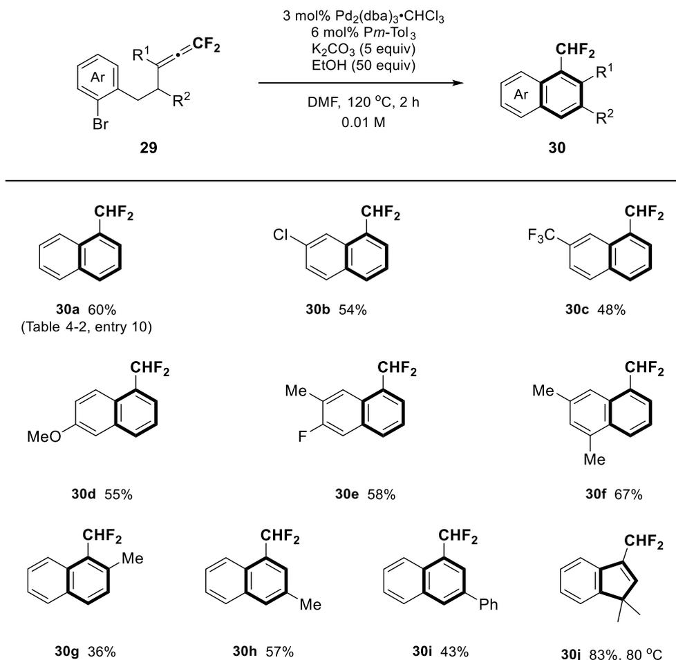
**Figure 4-3.** Synthesis of (Difluoromethyl)naphthalenes
