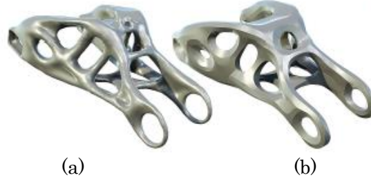
Figure 3-5 3D mesh data composed of developable surfaces [Stein_18]. (a) Original 3D data. (b) Developable polygon data.
