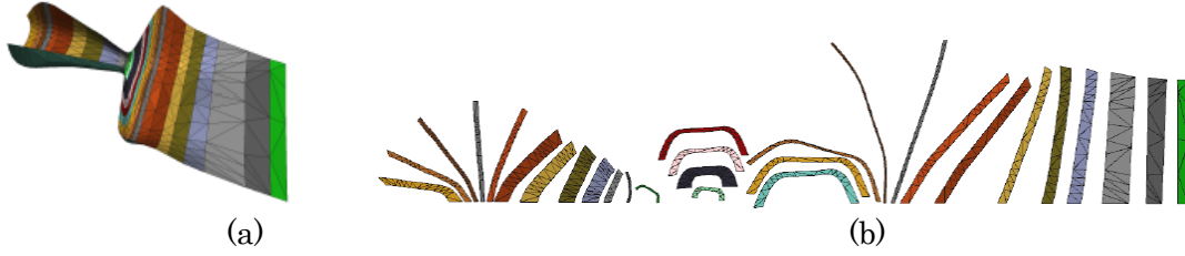
Figure 3-6 3D mesh data composed of developable strips [Liu_07]. (a) Triangulation of model. (b) Triangulation flattening.
